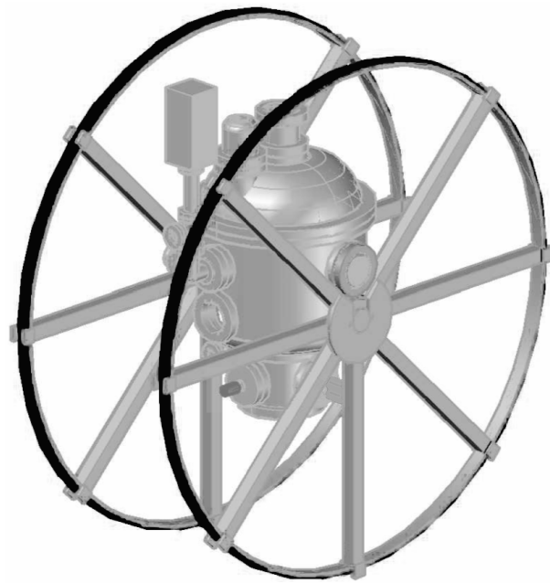
Figure 1.11: A view of the pair of Helmholtz coils on the COLTRIMS apparatus, in black. These are mounted to the camber roughly coaxial to the electron beam via an aluminum structure mounted to the electron gun feedthrough. The smaller coils (not pictured) mount to the same frame within the outer coils seen here.
