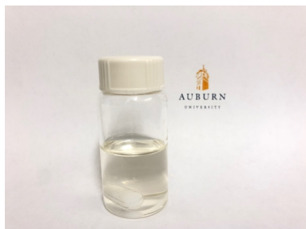
Figure 2.1 Uniform polymer solution formed in a glass vial
