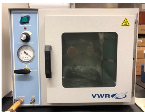
Figure 2.8 Image of VWR Thermo Scientific Vacuum Oven Model 6291
