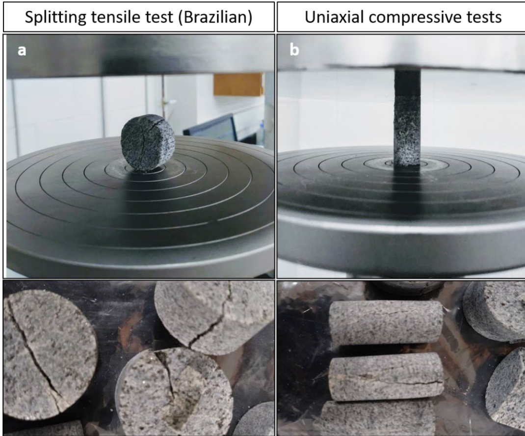
Figure 3.3. Fractured specimens after splitting tensile test (a) and uniaxial compressive test (b). Bottom figures show a zoomed view of samples.
