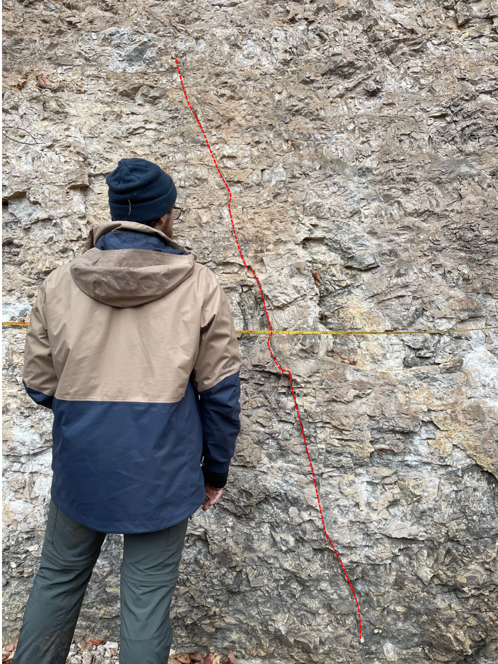
Figure 11: Highly brecciated chert beds surveyed at Boone 2. These fractures form a network of very small cuboidal blocks. Notice the long red fracture to the right of the researcher. Long, persistent fractures such as this are common in the chert beds of the Boone at this location. For reference, researcher is ~ 6 ft. tall.
