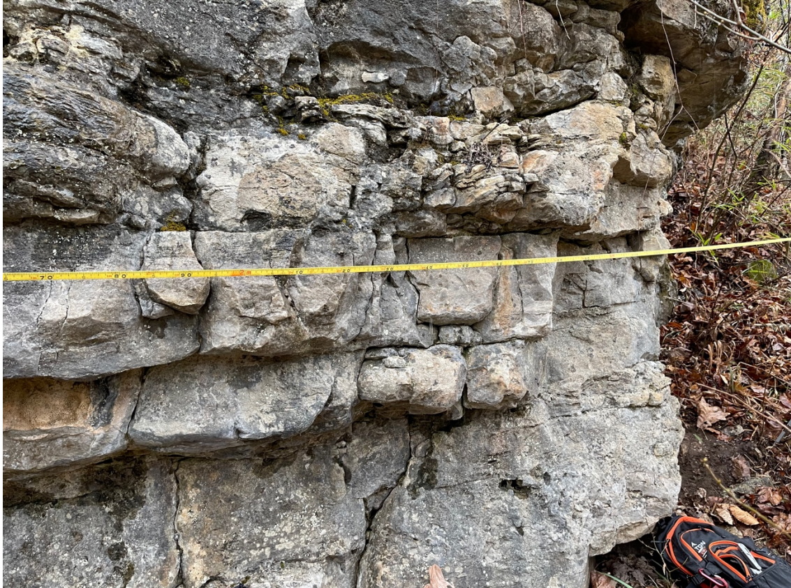
Figure 12: Fractures surveyed at Everton 2. Fractures at locations of Roark Bluff often do not cross bedding planes. Here the bedding plane is gently dipping and can be seen to have a somewhat wide aperture, which is one of the main reasons the bedding plane is considered to contribute to instability in many areas.
