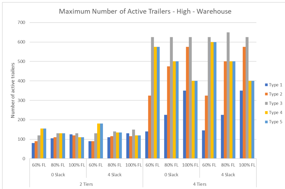
Figure 4.10: Maximum number of active trailers for each design point per trailer type (1,2,3,4, & 5) when the demand pattern is high with warehouses.
