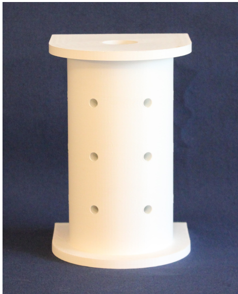
Figure 2-14 - SISO - Nozzle with Radial Perforations - Prototype
