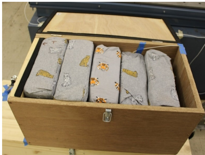
Figure 3-15 - MIMO Test Box - Inner Box with Smaller Prototype
