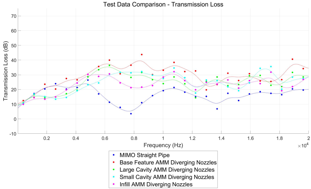
Figure 3-81 - MIMO - Diverging Configurations - Transmission Loss Comparison
