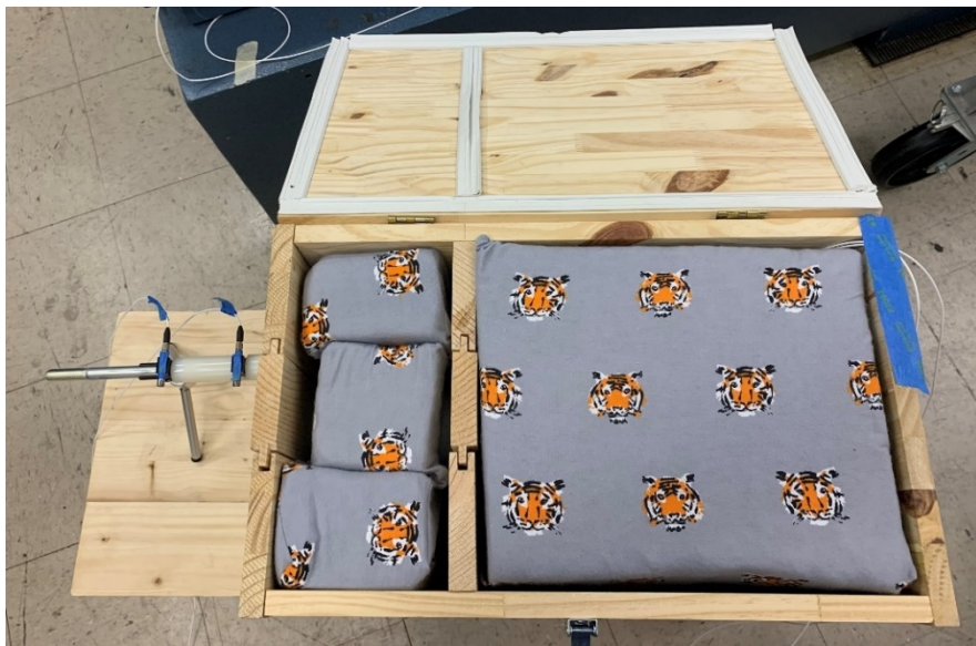
Figure 3-11 - SISO - Test Box - Inner Box with Insulation View
