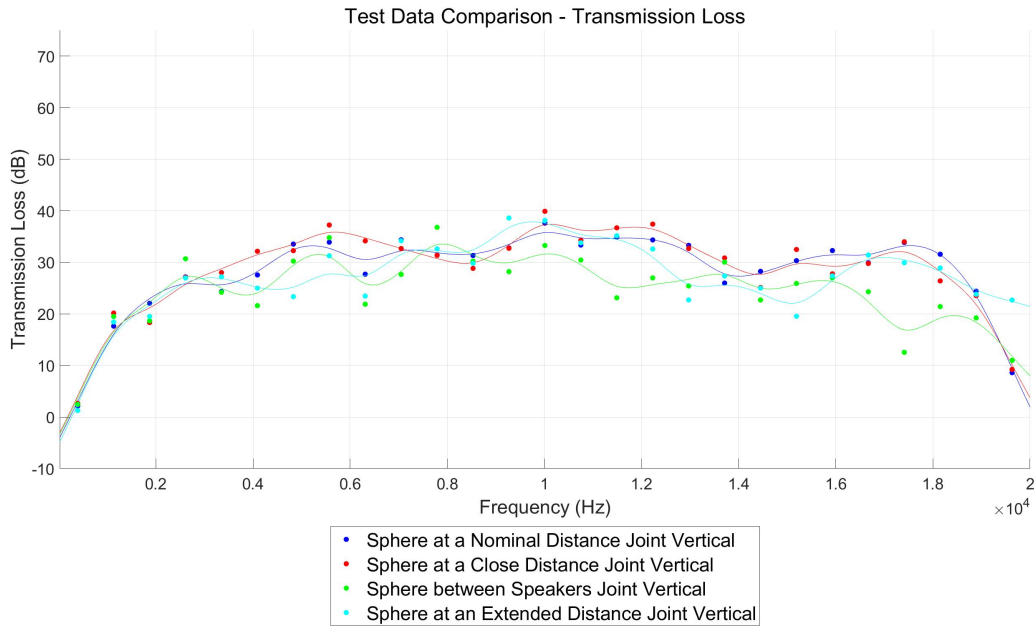
Figure 3-104 - AMM Sphere - Test - Joint Vertical - Transmission Loss Comparison
