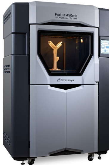
Figure 2-4 - Stratys Fortus 450 Gen2 Additive Manufacturing Machine [36]
