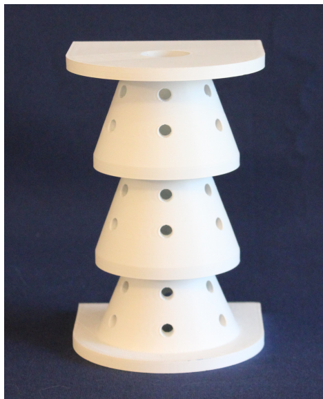
Figure 2-29 - SISO - Series of Diverging Nozzles with Radial and Axial Perforations and a Constricted Opening at the Output Plane - Prototype
