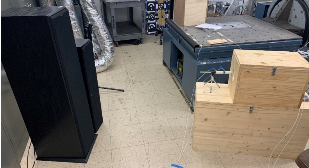
Figure 3-12 - SISO - Test Setup - Speakers and Test Box
