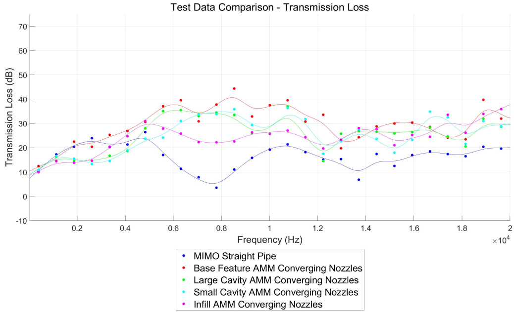
Figure 3-80 - MIMO - Converging Configurations - Transmission Loss Comparison
