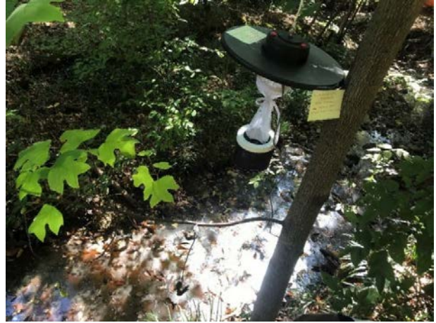
Figure 3 Mosquito trappers used to trap mosquitoes at Auburn in Alabama. (Left panel): CO 2 -baited BG-2-Sentinel Mosquito Trap. (Right panel): UV light baited New Standard Miniature Mosquito Trap.
