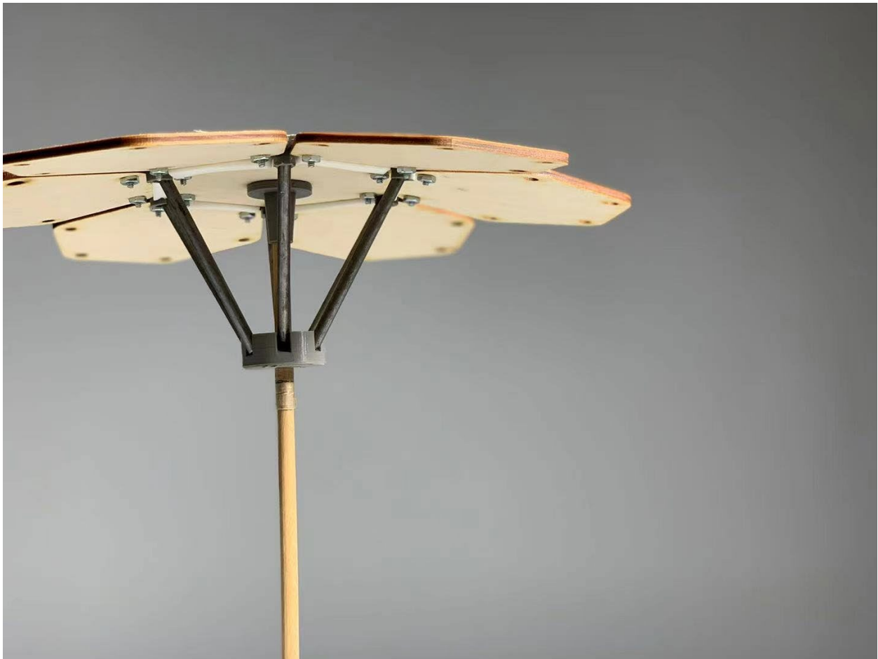
Figure 4.5.3 Re-prototype Solar Module Top Support
