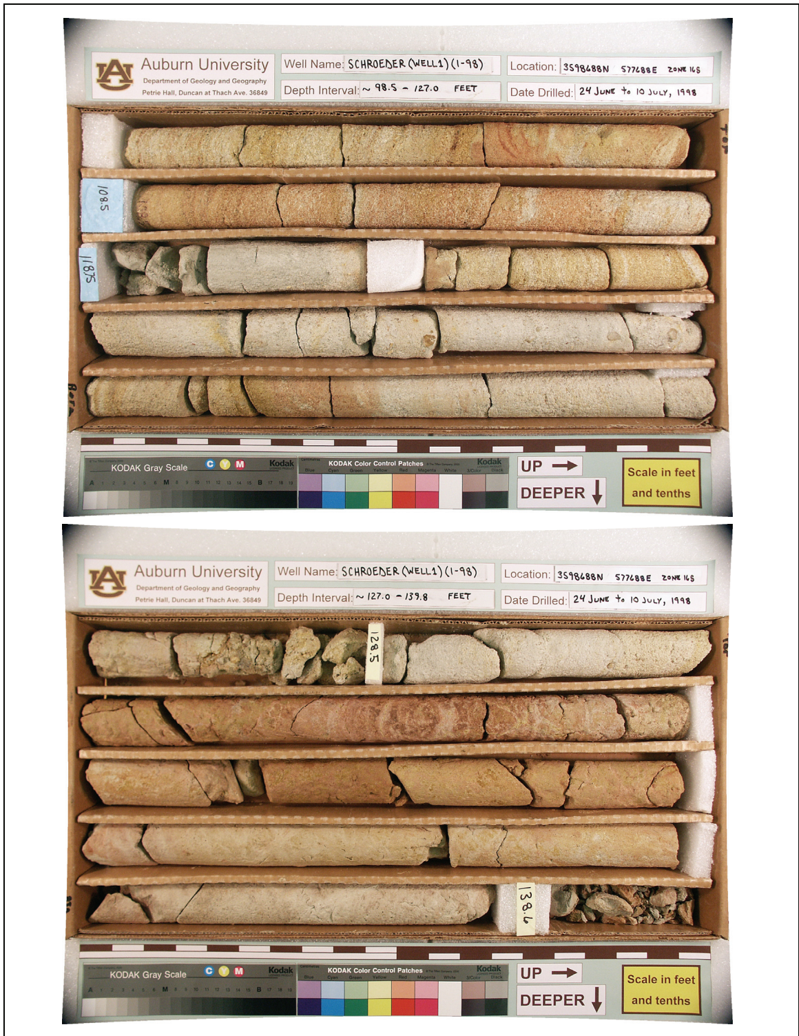
Figure A - 2. Boxes 1 (top) and 2 (bottom) of drill core 1-98.
