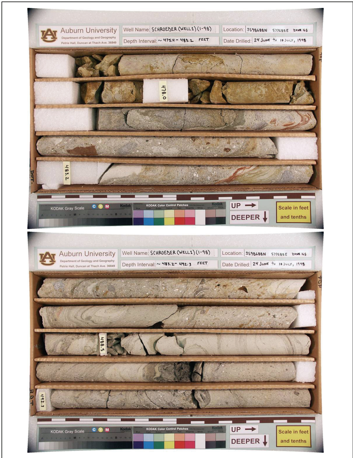
Figure A - 18. Boxes 33 (top) and 34 (bottom) of drill core 1-98.
