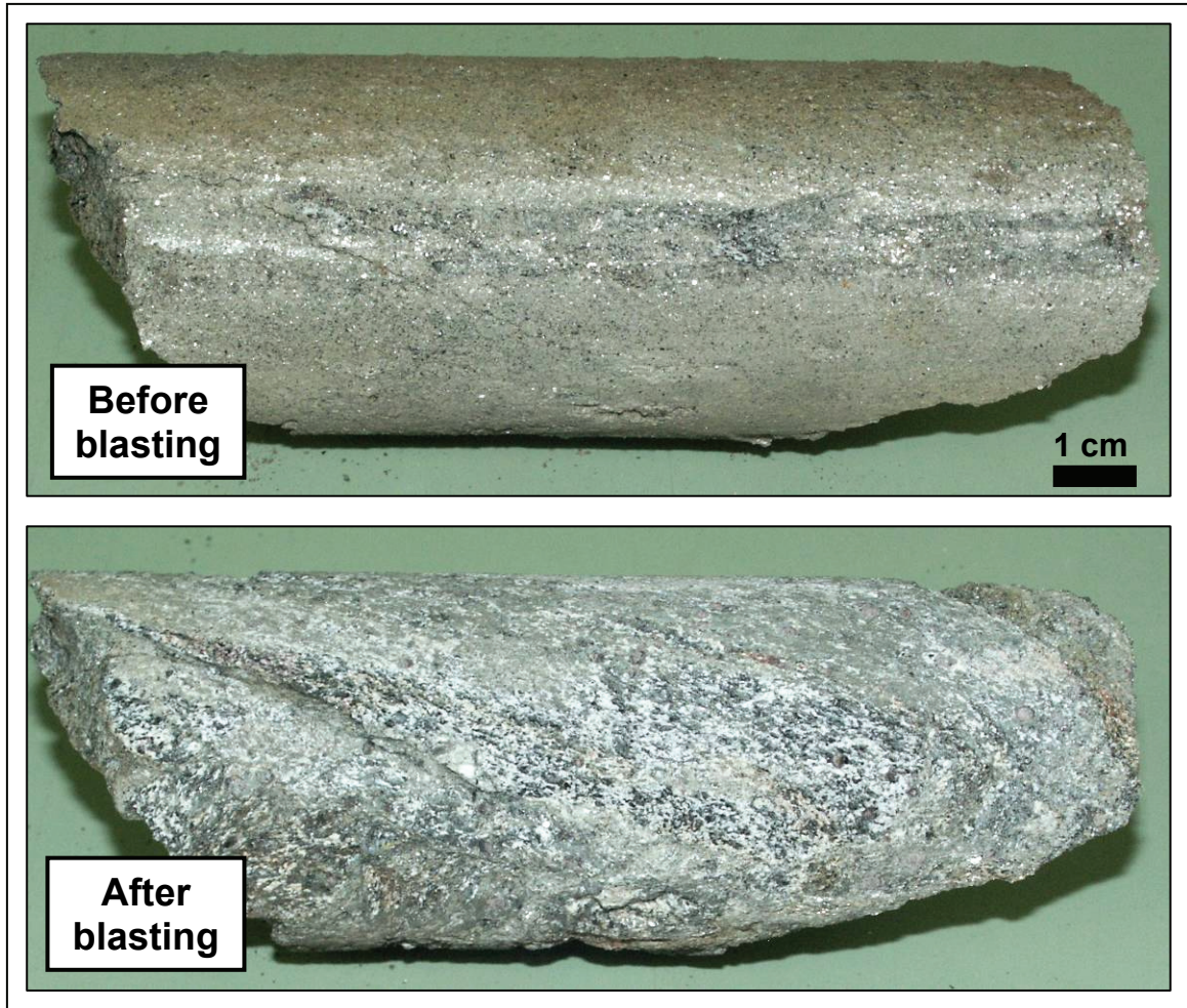
Figure 53. Example of crystalline drill-core facies before and after cleaning by abrasive (sand) blasting. Cleaning exposed the pre-impact metamorphic fabric within this core piece. Although the crystal faces of the mineral grains were mildly etched by the blasting process, etching was no more destructive than that caused by the drilling process itself.
