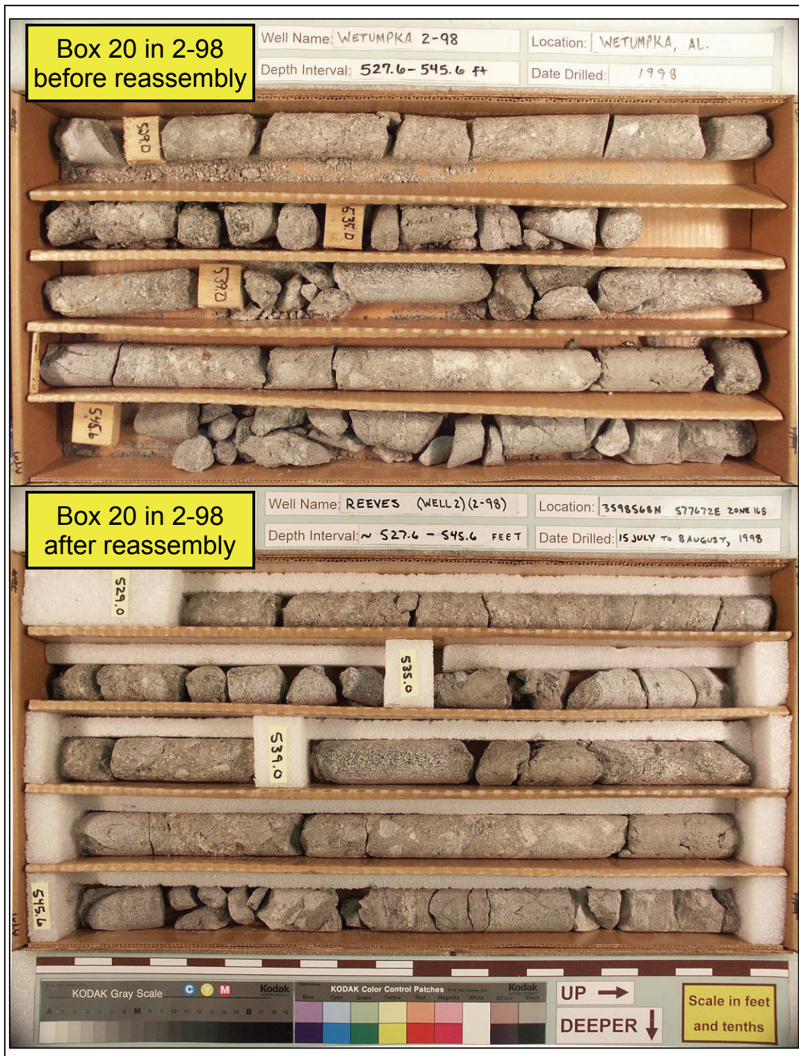
Figure 55. Example of boxed drill core before and after reassembly. The same box is depicted in each photo.
