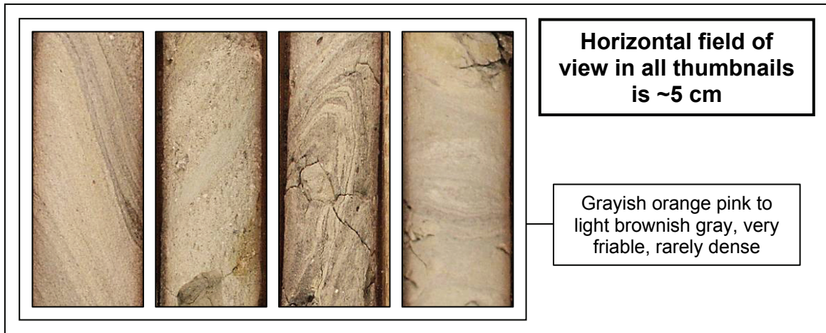
Figure 60. Representative examples of various Bedded Sandstone lithofacies.
