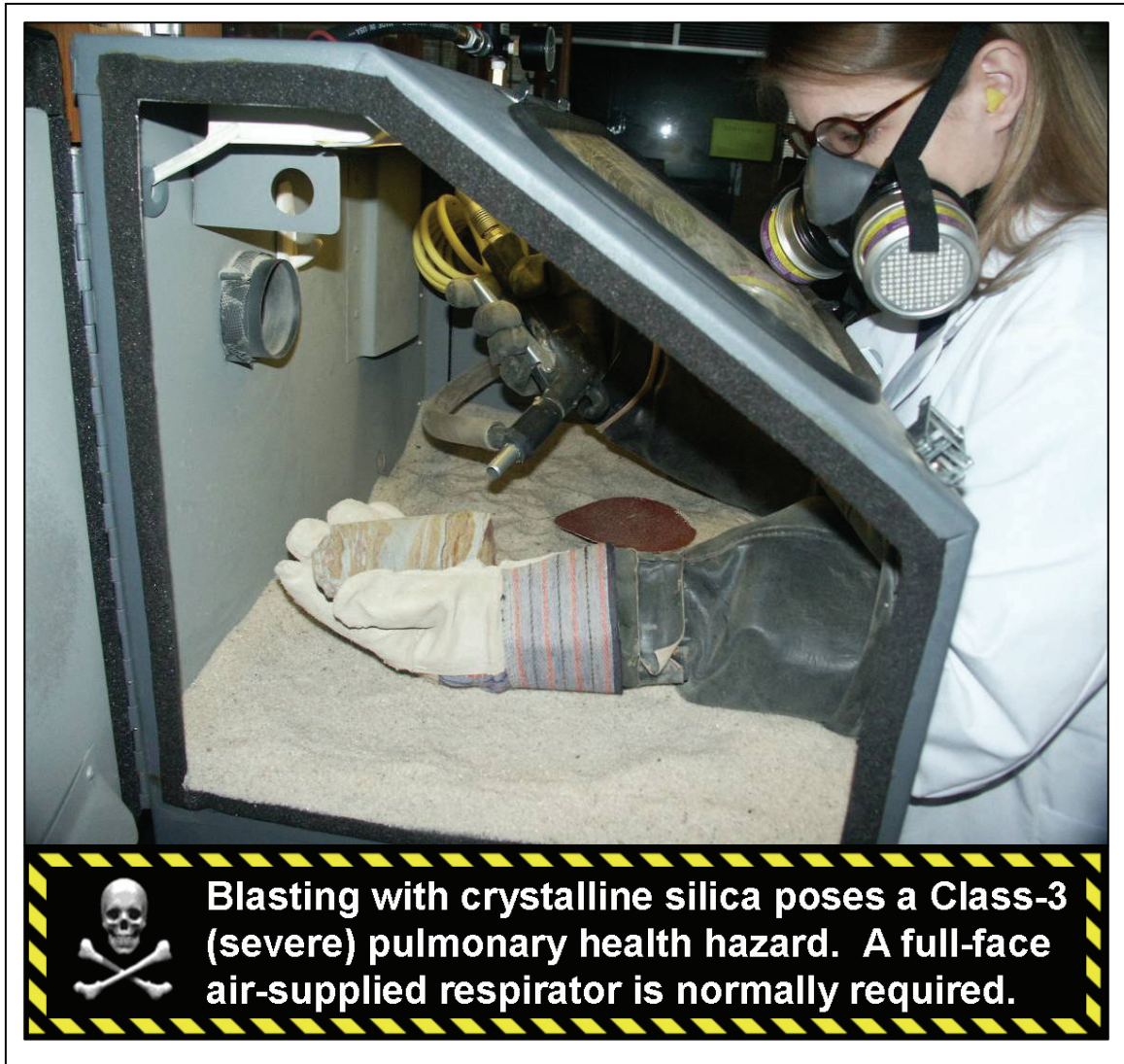
Figure 37. Blasting procedure ( simulated for purpose of photo) showing operator wearing protective gear as described in text. Blasting must be done only with the cabinet doors fully closed. Notice the sand hopper/reservoir is filled up to where sand completely overtops the screened work surface (not visible). This provides a soft bed for the core pieces, and helps keep the blasting gun well fed with sand.
