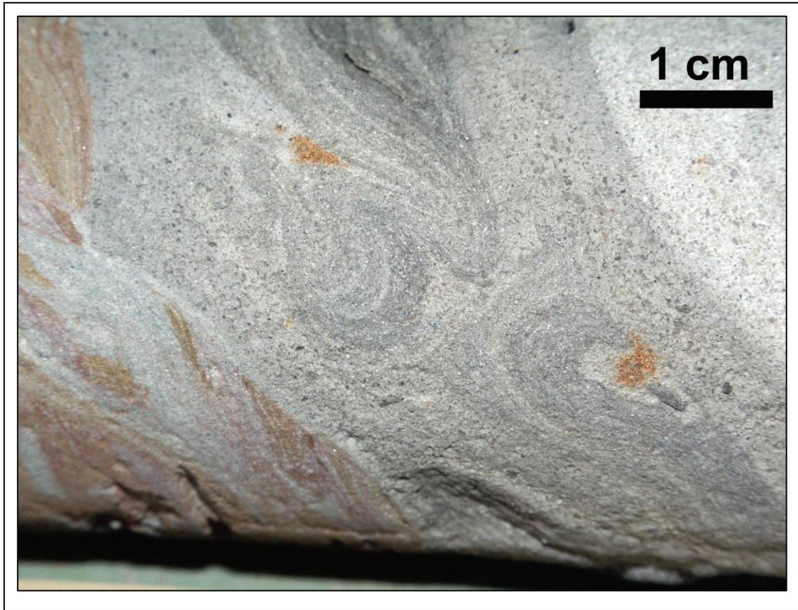
Figure 54. Close-up of millimeter-scale details brought out and left undamaged by abrasive (sand) blasting of a drill core piece containing fluidized and plastically deformed sands and muds. Such details would have been obliterated or at least strongly altered by other cleaning methods.
