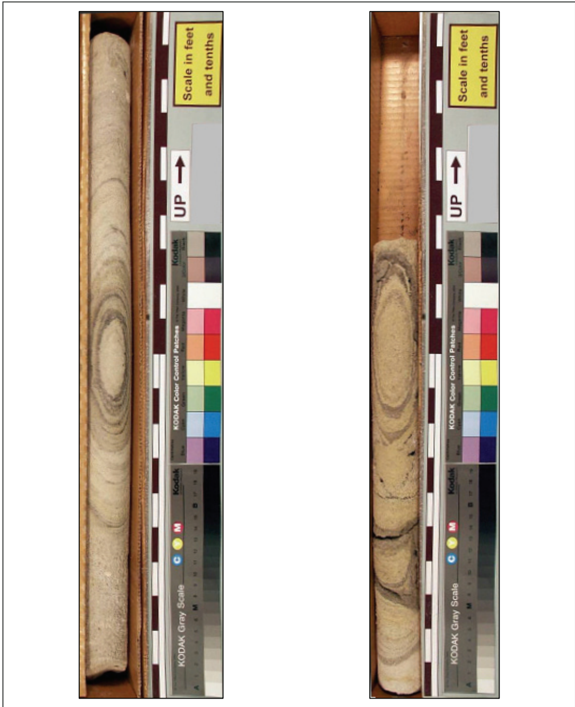
Figure 31. Two examples of bull's-eye patterns in drill core from the Wetumpka impact structure. The patterns wrap around much of each core leg. Both photos are of core legs taken from 1-98 (the Schroeder drill hole) at depths of 121.5 m (left) and 181.2 m (right).
