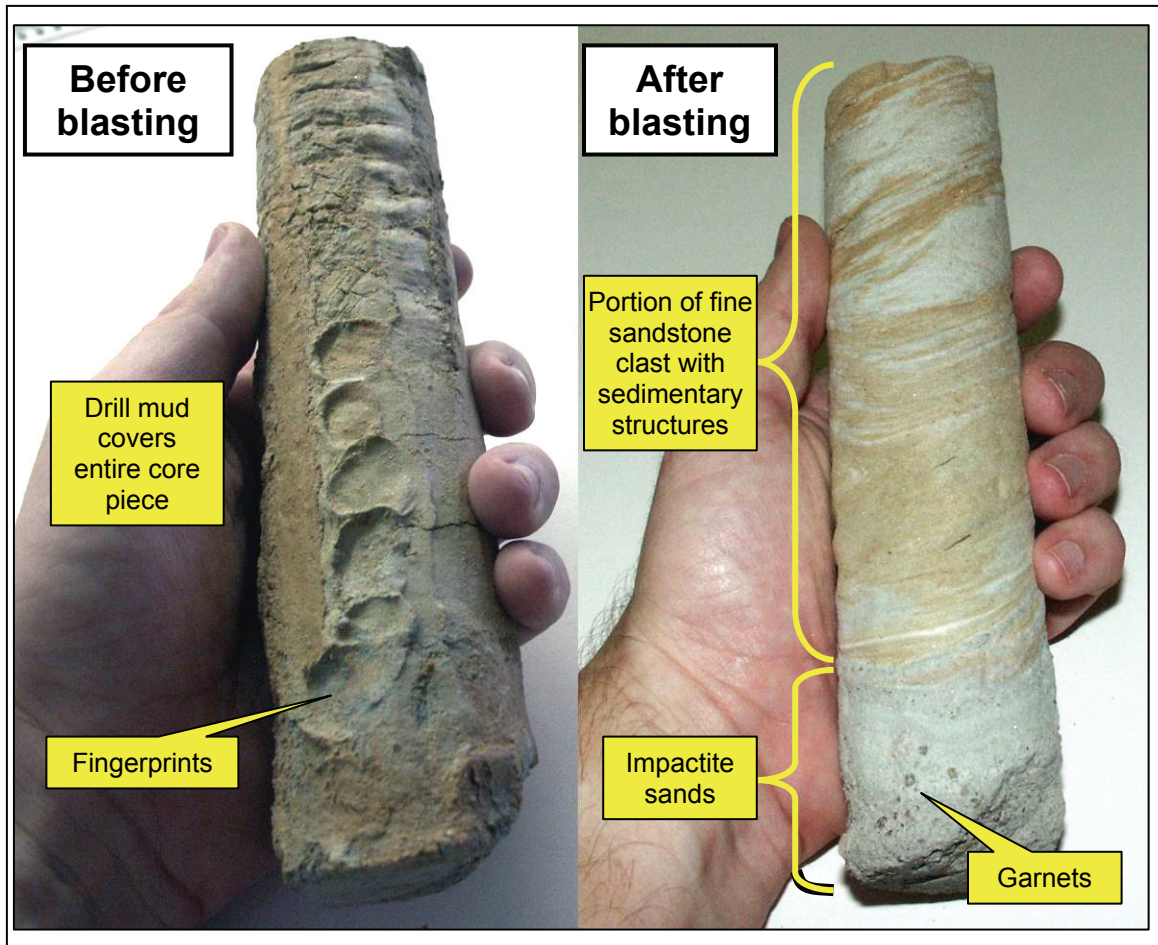
Figure 52. Example of sedimentary drill-core facies in especially poor condition before and after cleaning by abrasive (sand) blasting. Cleaning not only exposed immediately recognizable small-scale sedimentary structures and millimeter-scale garnets, but also revealed that what originally appeared to be a core piece of homogeneous lithology is actually composed of two distinct lithofacies. Modified from Johnson et al. (2006).
