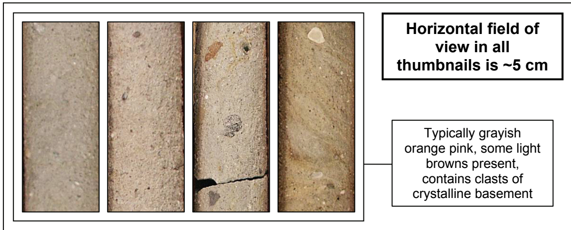
Figure 64. Representative examples of various Structureless Sandstone lithofacies.
