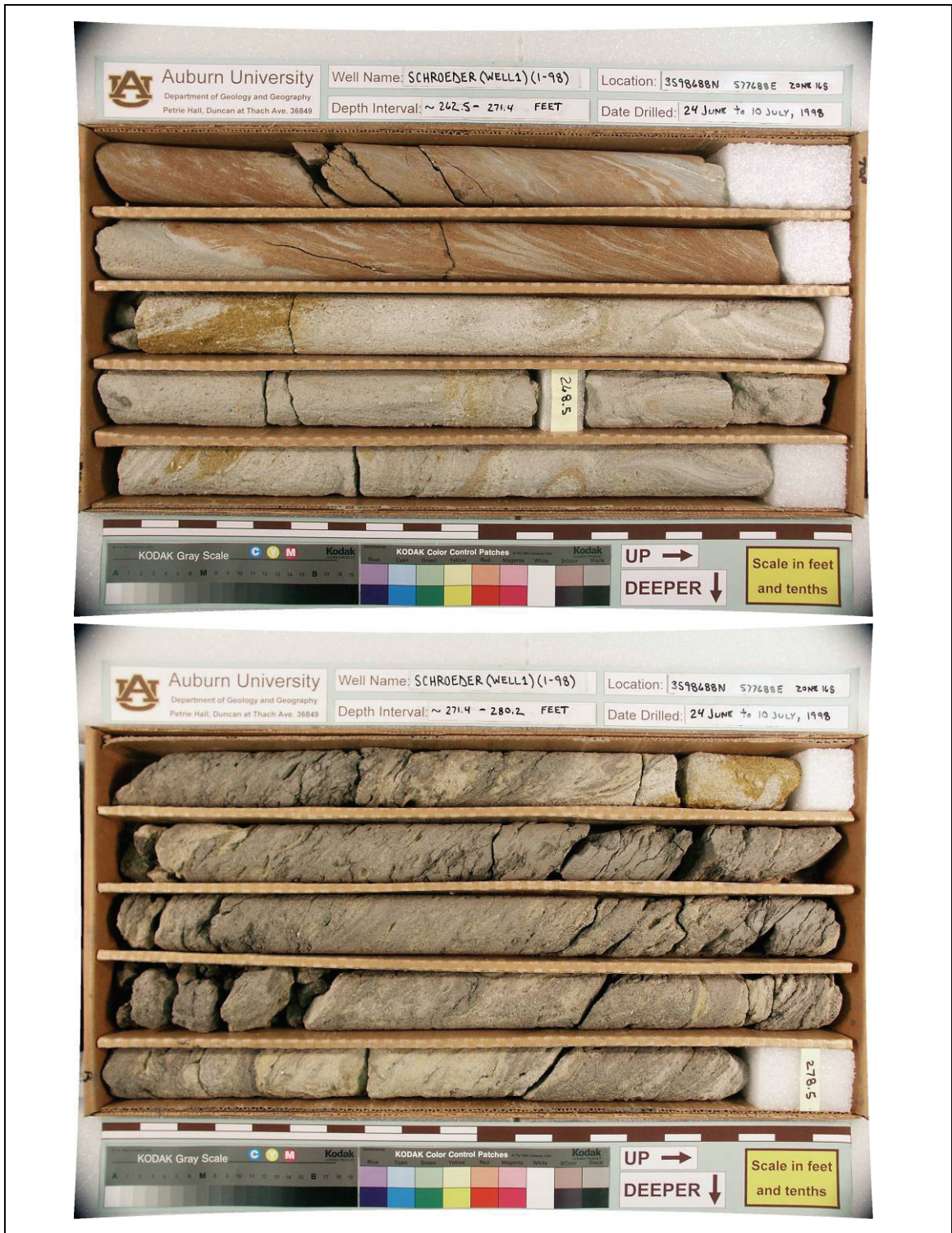
Figure A - 7. Boxes 11 (top) and 12 (bottom) of drill core 1-98.
