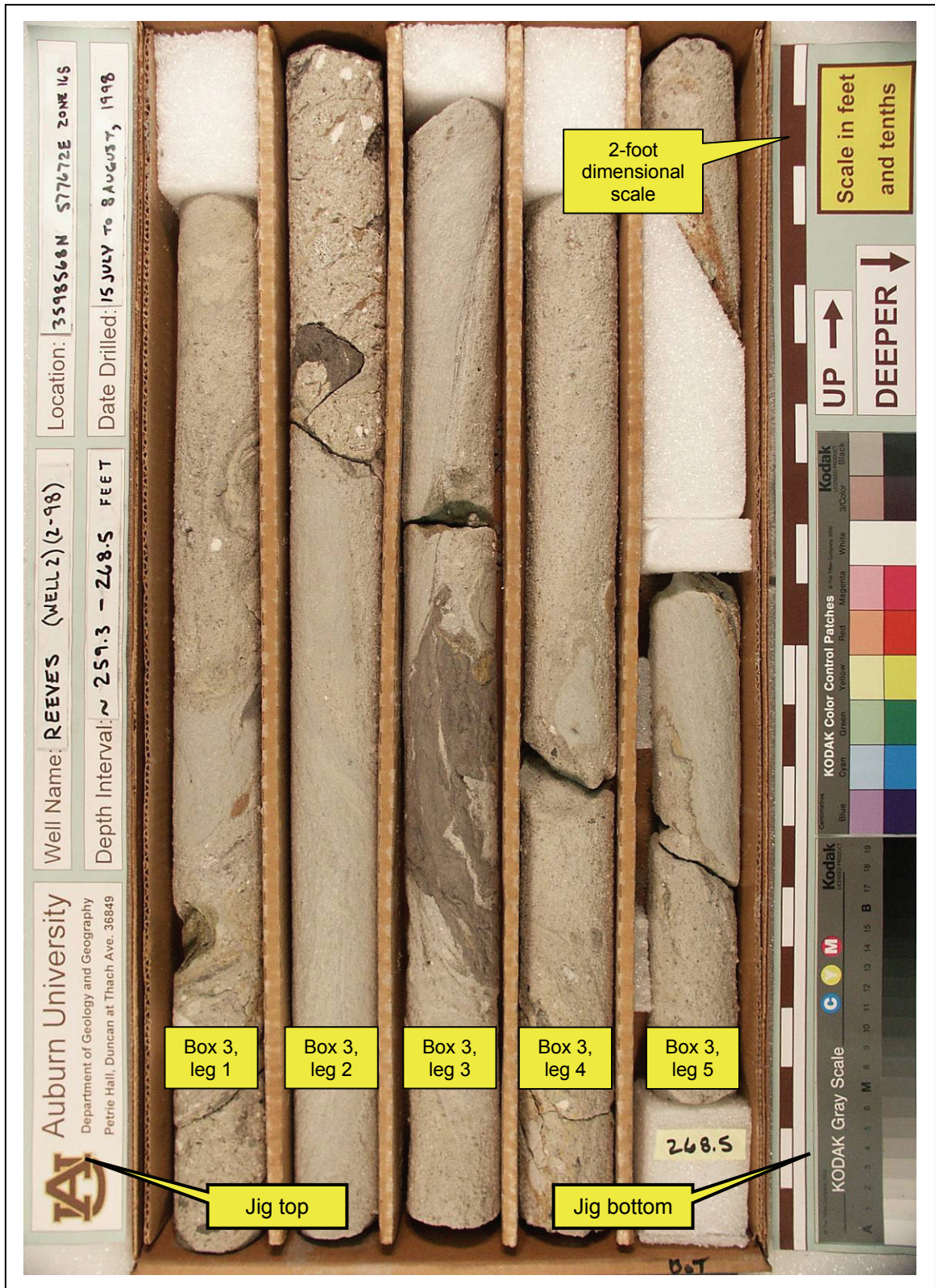
Figure 40. Boxed drill core resting in the jig with relevant data specific to the box.
