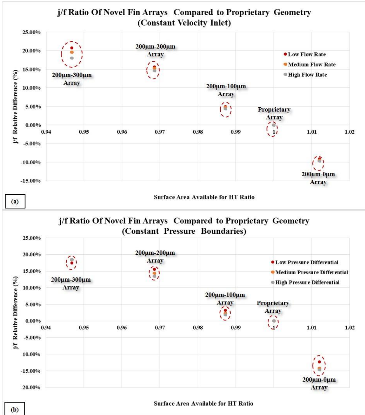
Figure 58: Comparison of j/f_{app} using (a) Constant Velocity Boundary and (b) Constant Pressure Differential Boundary
