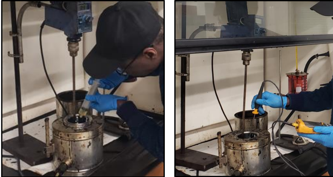
Figure 3.3: Preparation of recycled binder blends (a) Addition of RAs (b) checking temperature
