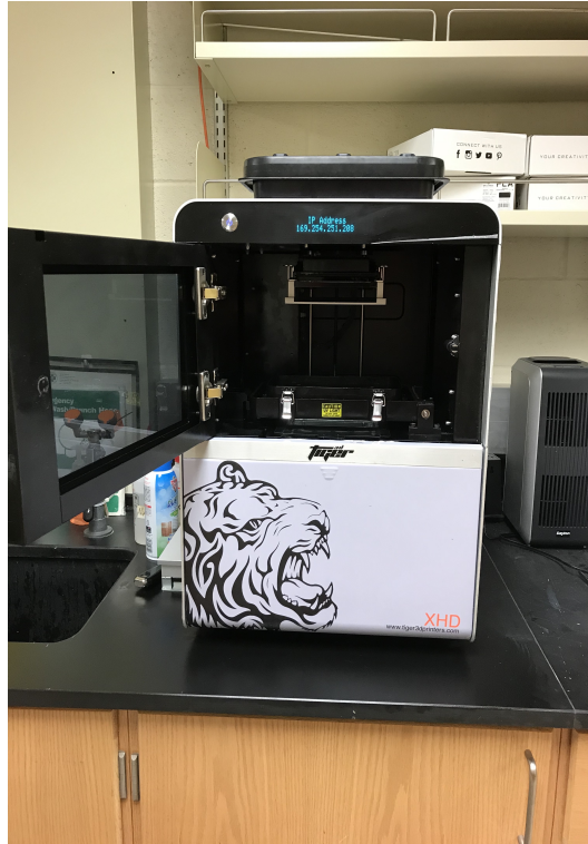
Figure 4.17: A picture of the Tiger printer XHD made by Romanoff with its door open revealing the build plate and resin reservoir.
