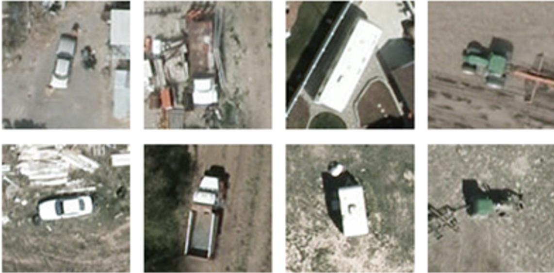
Figure 6.1: Vehicle Detection in Aerial Imagery (VEDAI) sample data showing different vehicles in different orientations from an overhead visible sensor.
