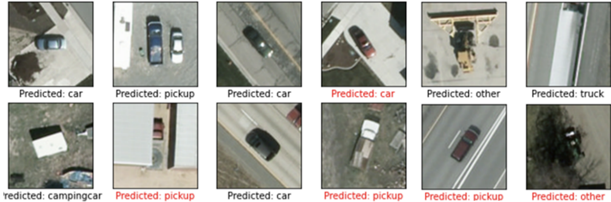
Figure 6.4: Randomly selected samples from the dataset with predictions from the Visible Model. The black predictions are correctly classified images and the red predictions are the incorrect predictions with the selected class.
