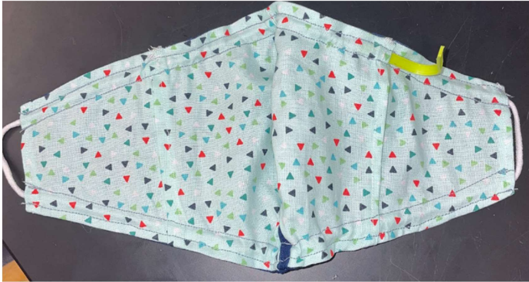
Figure 60: Prototpye-5 with silver nanoparticle coating
