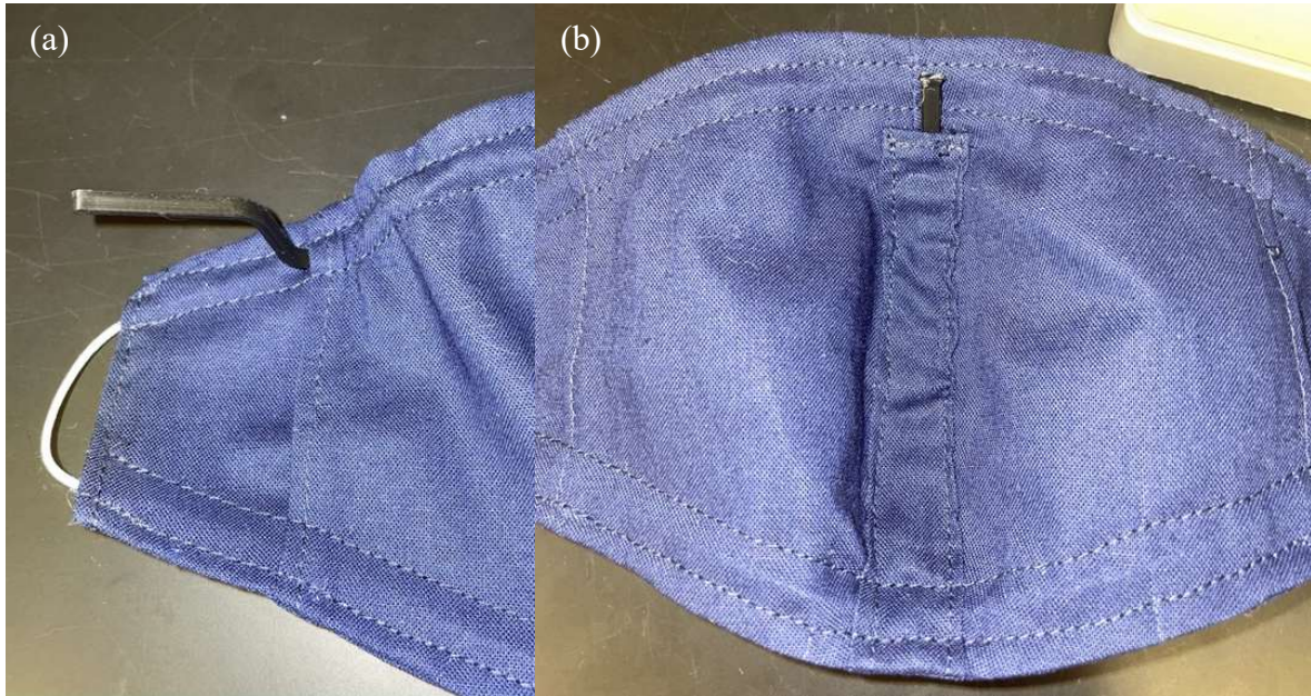
Figure 46: Fourth prototype - brace insert channels (a) at nose and (b) at mouth
