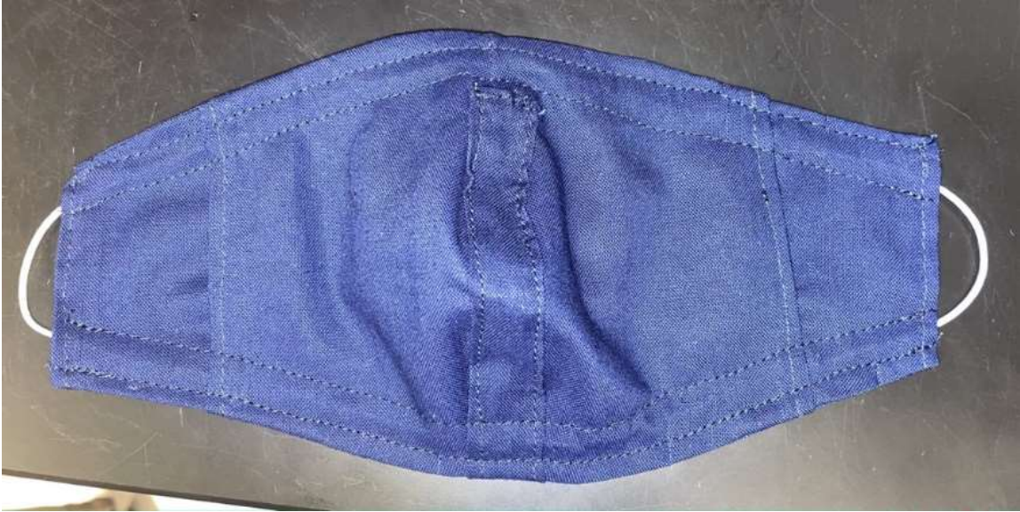
Figure 47: Fourth prototype - further extended sides for ear loops
