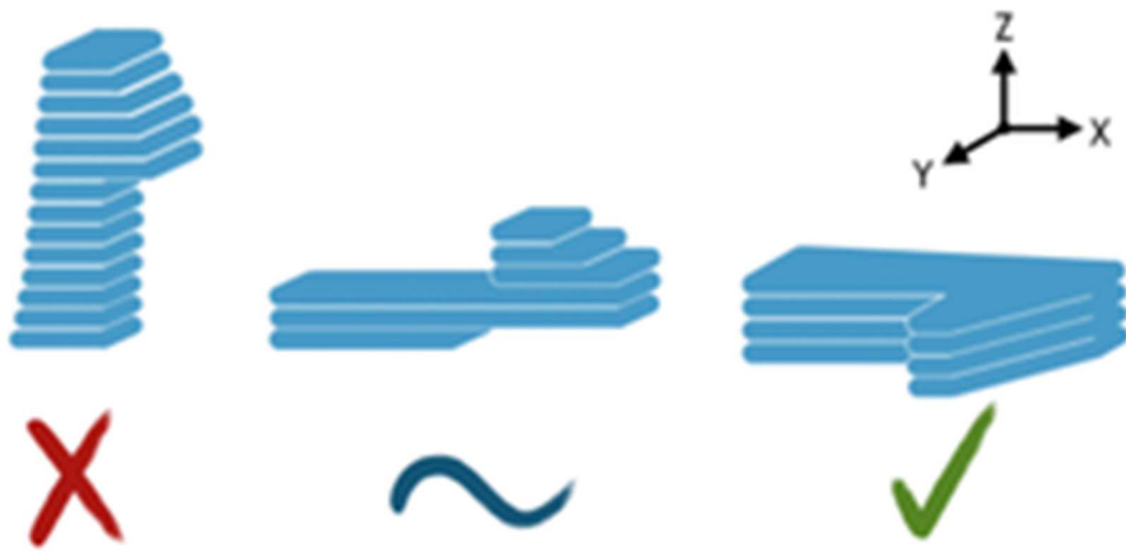
Figure 40: Layer lines related to 3-D printed snap fits [28]
