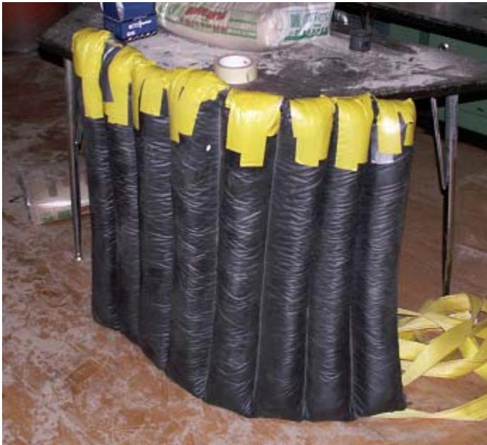
Figure 22 Center Connected Bags Filled with Vermiculite
