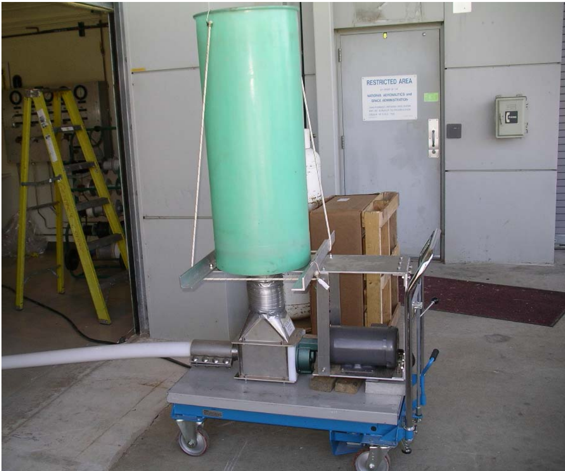
Figure 26 Screw Conveyor System- Image shows a motor attached to helical screw running inside the tube. The container is filled with vermiculite. When vermiculite pours into the screw it is carried through the pipe and into the bags.
