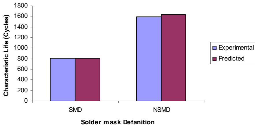
Figure 3.9: Effect of solder mask definition on thermal fatigue reliability of Flex-BGA packages
