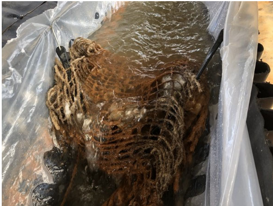
Figure 56 Longevity test clear water introduction.
