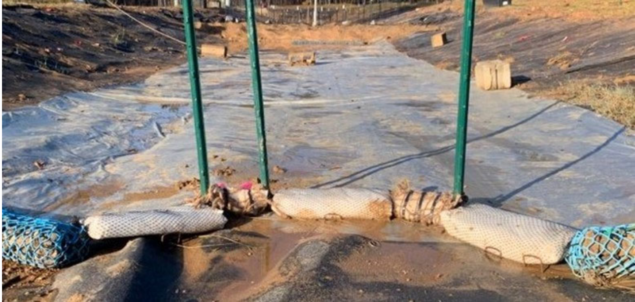
Figure 70 Flocculant introduction in testing channel (Schussler 2022).
