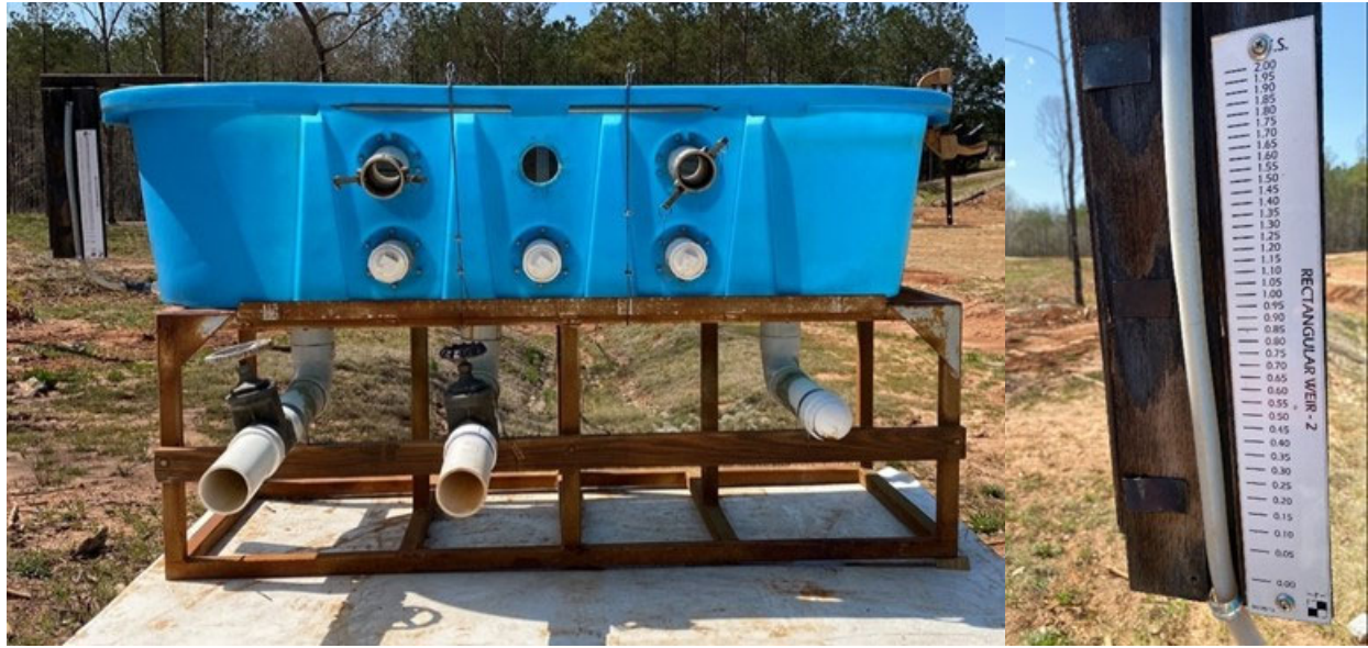
(a) the backside of the equalizing flow tank (b) flow control guide Figure 46 Equalizing tank system for flow introduction.
