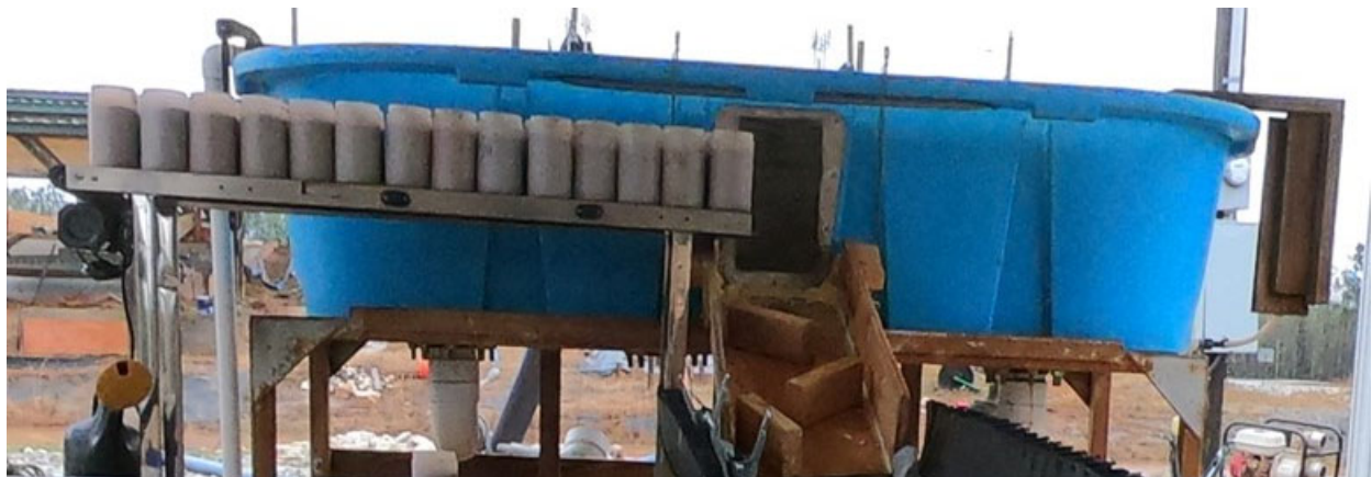
Figure 48 Sediment introduction setup.
