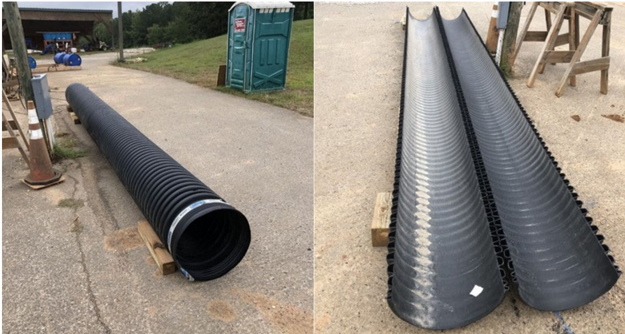
(a) double-wall corrugated smooth interior HDPE pipe
