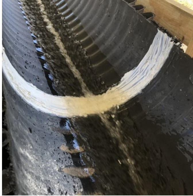
Figure 43 Flume mid-section hydraulic jump test.
