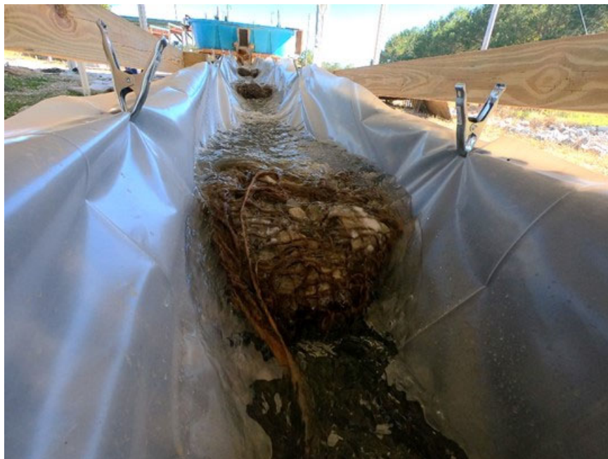
Figure 51 Clearwater flume experiments with a granular form.
