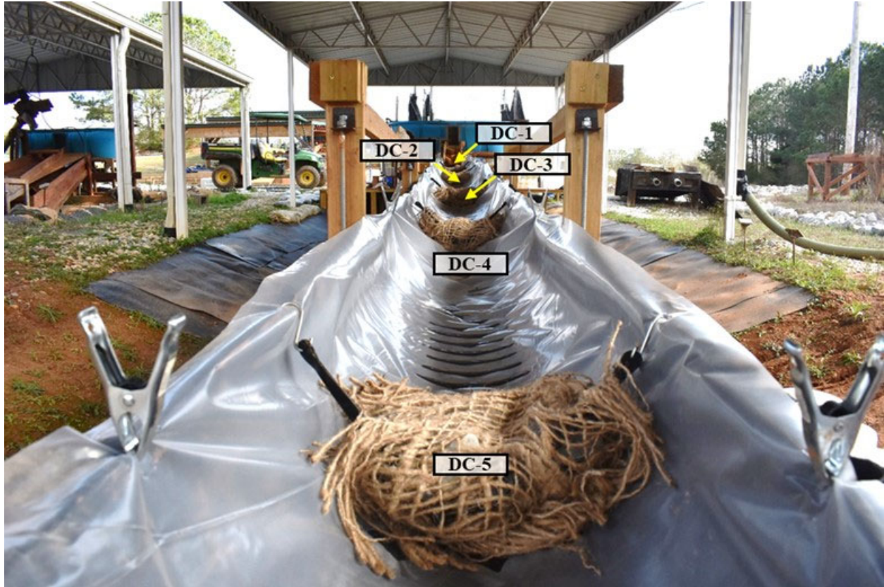
Figure 49 Scaled-down rock ditch checks in the flume.
