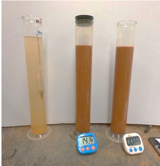
Figure 17 Hydrometer testing setup.
