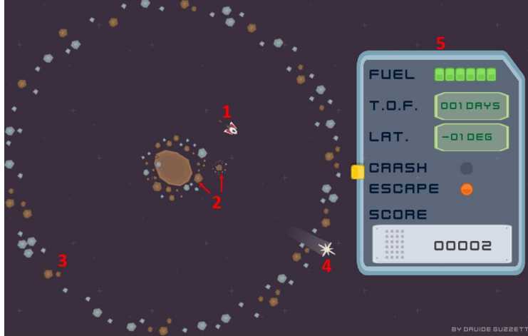
Figure 6.2: The interface for the real time flight simulator that visualizes spacecraft motion (1), primary and secondary asteroids (2), outer ring representing the termination criteria for escape (3), apparent sun position (4), and the interface dashboard (5).
