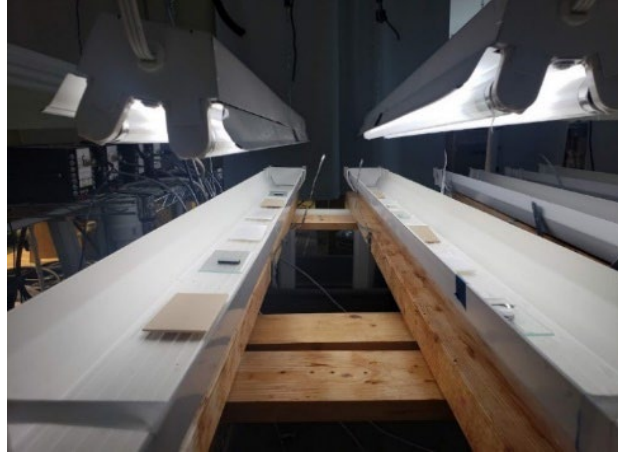
Figure 4.4 Substrate surfaces (glass, PTFE, and PLA) in the photobioreactor prior to cultivation.
