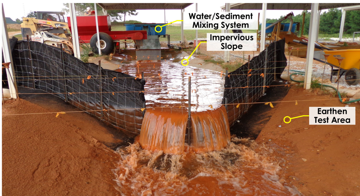
Figure 2.3. Photo of ditch check test apparatus.
