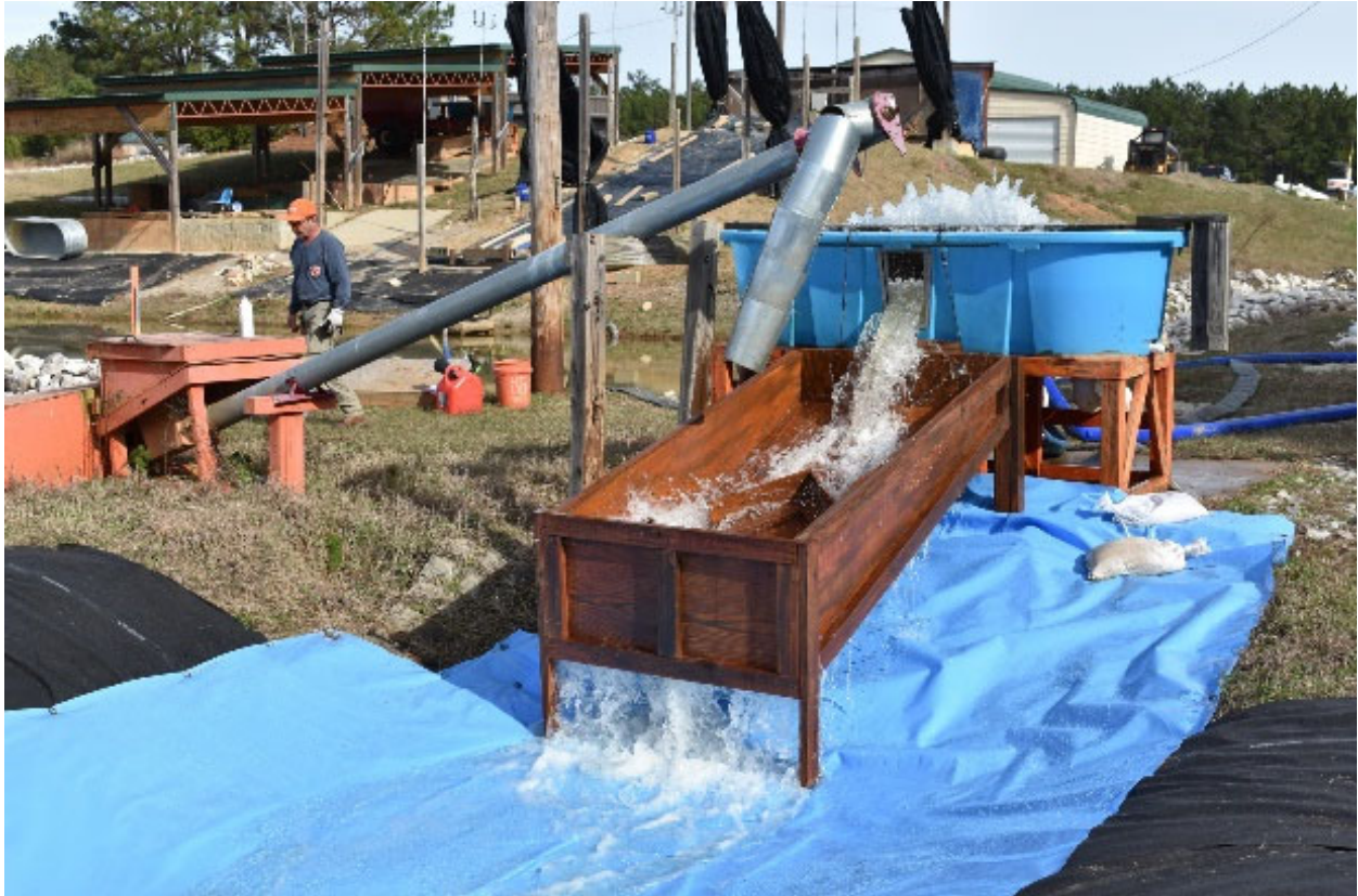
Figure 7.2. Water introduction system for post-construction basin.
