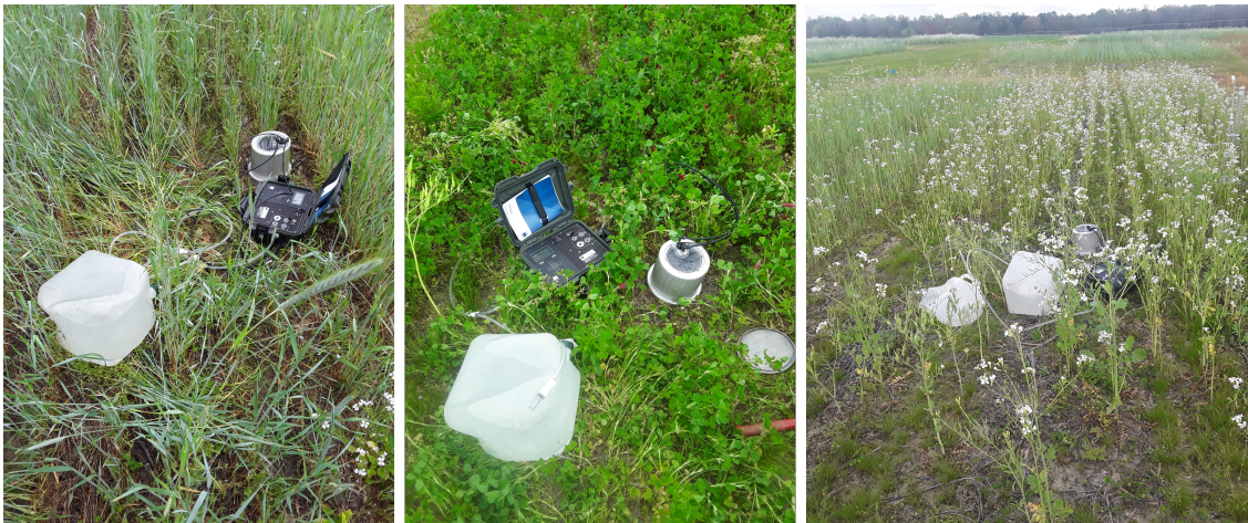
Figure 2.4: Saturo measurements in the radish, cereal rye, and crimson clover cover crop plots during spring.
