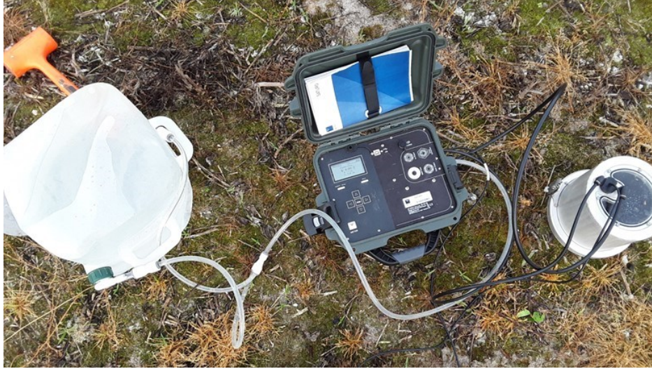
Figure 2.6: Saturo and its components, metal ring, pressure chamber, water supply tank, and the control unit.
