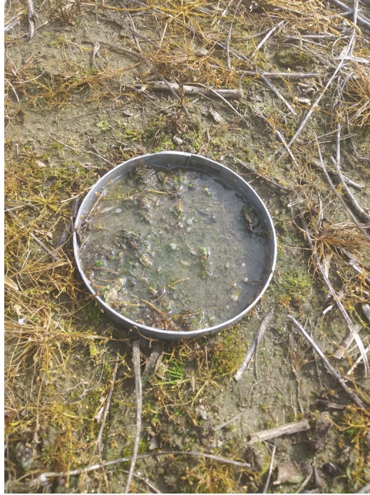
Figure 2.10: Ring infiltrometer in one of the points where data was collected during 2021 for the BEST-1K.
