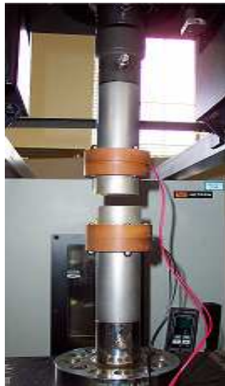
Figure 4.2 Through-plane conductivity measurement on INSTRON 4505 testing device
