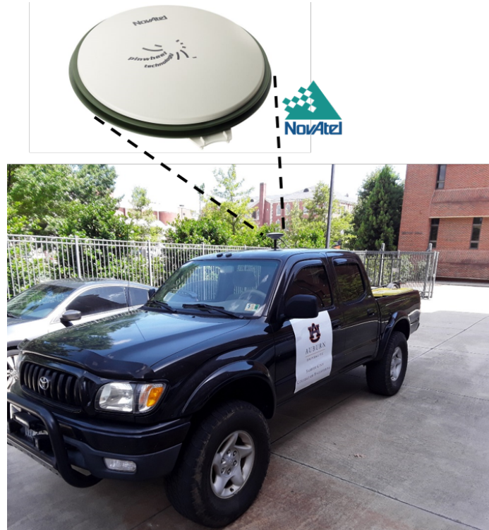
Figure 4.6: Research Vehicle Setup for Dynamic C/N_0 Data Collection
