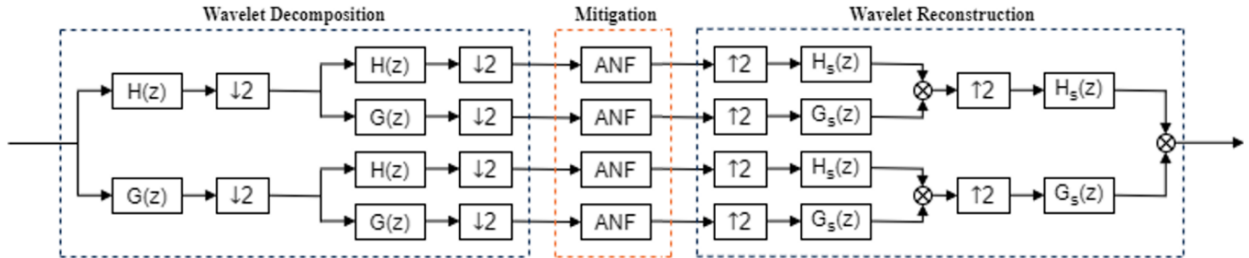
Figure B.4: Level 2 Wavelet Decomposition and Reconstruction Architecture
