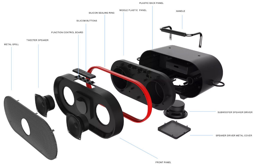
Figure 5.9 Exploded View of Waterproof Speaker (Huang, 2022)
