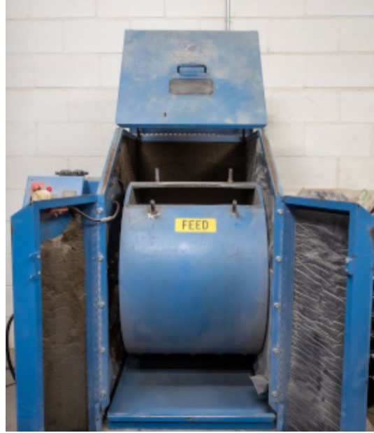
Figure 7. Cantabro Testing Apparatus
