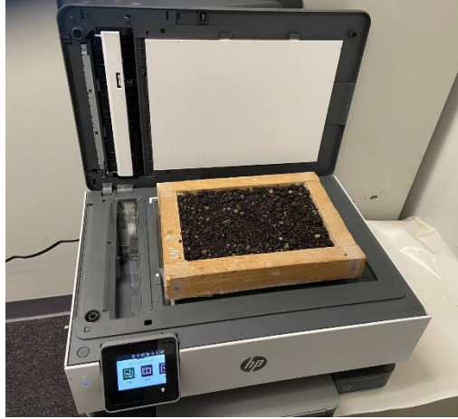
Figure 8. Grayscale Image Analysis Apparatus
