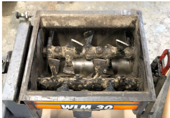
Figure 5. Wirtgen Pugmill Utilized in Pretreatment
