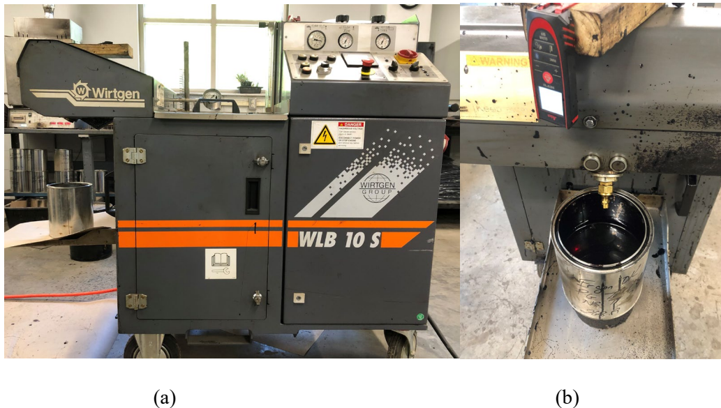
Figure 3. Foaming Optimization Setup: (a) Wirtgen WLB 10s Laboratory Foaming Unit and (b) Laser Distance Meter
