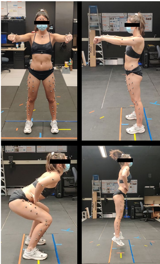
Figure 8: This figure shows a subject during calibration and during phases of the repeated vertical jump. Top-Left) Frontal calibration view. Top-Right) Side calibration view. Bottom-Left) Subject at maximum knee flexion during a vertical jump. Bottom-Right) Subject at peak of vertical jump.
