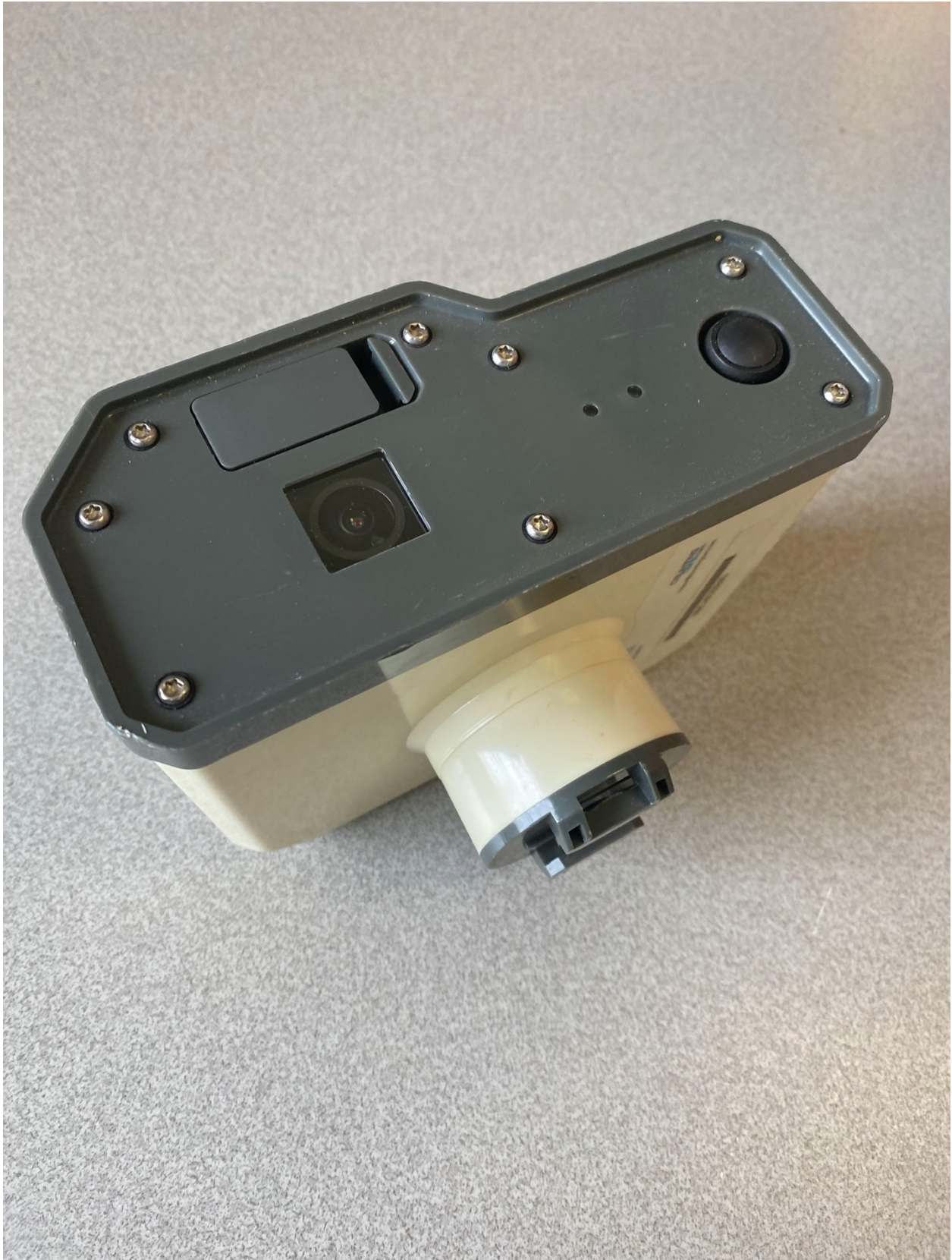
Figure 3 A Portable Camera used to record Illegal Left Turns
