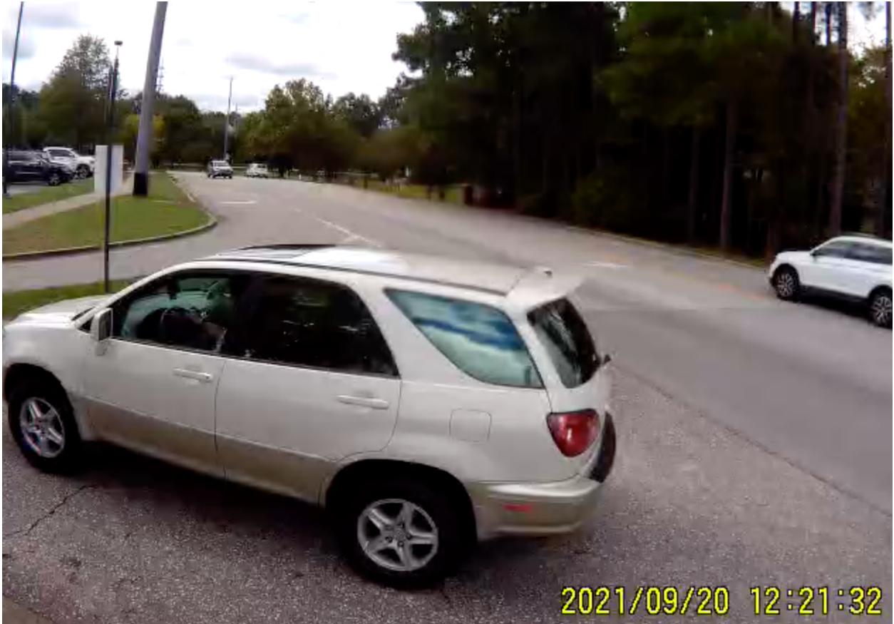
Figure 26 Motorist Driving on Wrong Side of Channelizing Island at Wire Road Location
