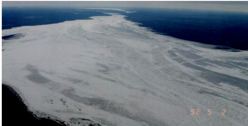
Figure 2.10 Thermal break-up of ice cover because of snowmelt on the ice cover (photo by F. Hicks)
