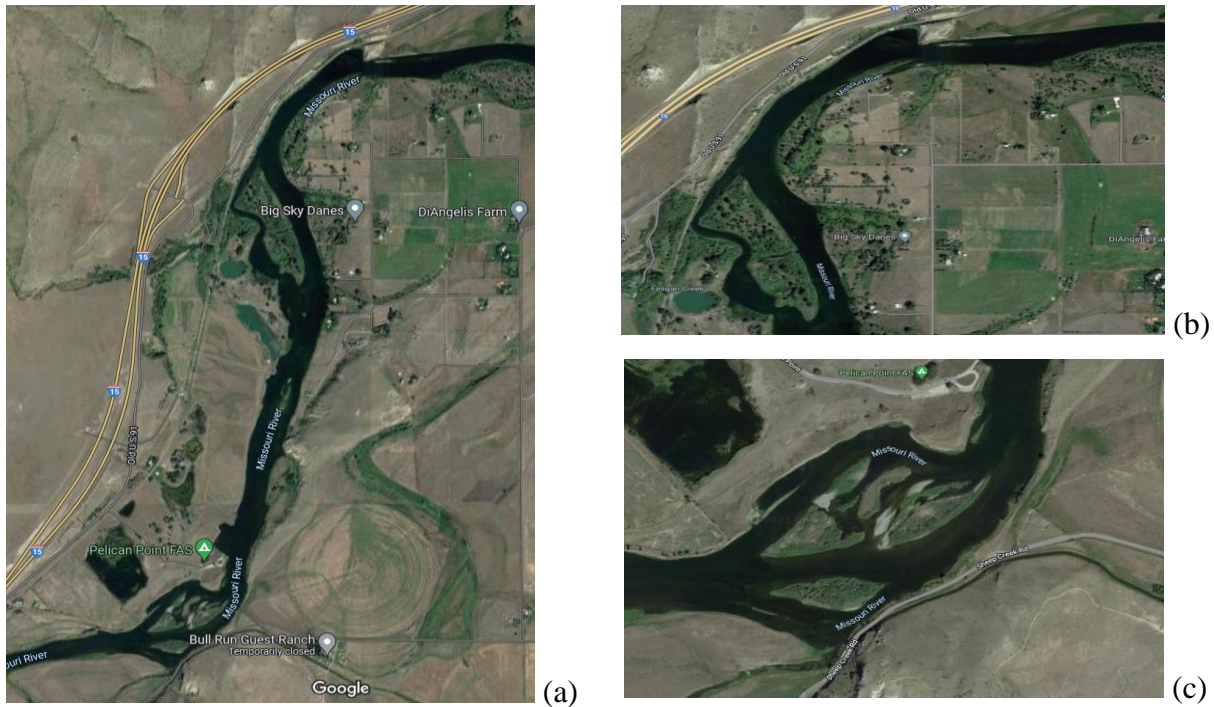
Figure 6.15 Google Earth image of Missouri River showing the ice bridging locations. (a) Portion of Missouri River with narrow width, and bifurcation of river with small higher elevation land mass in the river. (b) Enlarged portion of (a) showing the bifurcation portion of the river and immediately a constriction downstream. (c) Portion of the Missouri River with trifurcation of the river with small land masses in the river serving as constriction to the flow.
