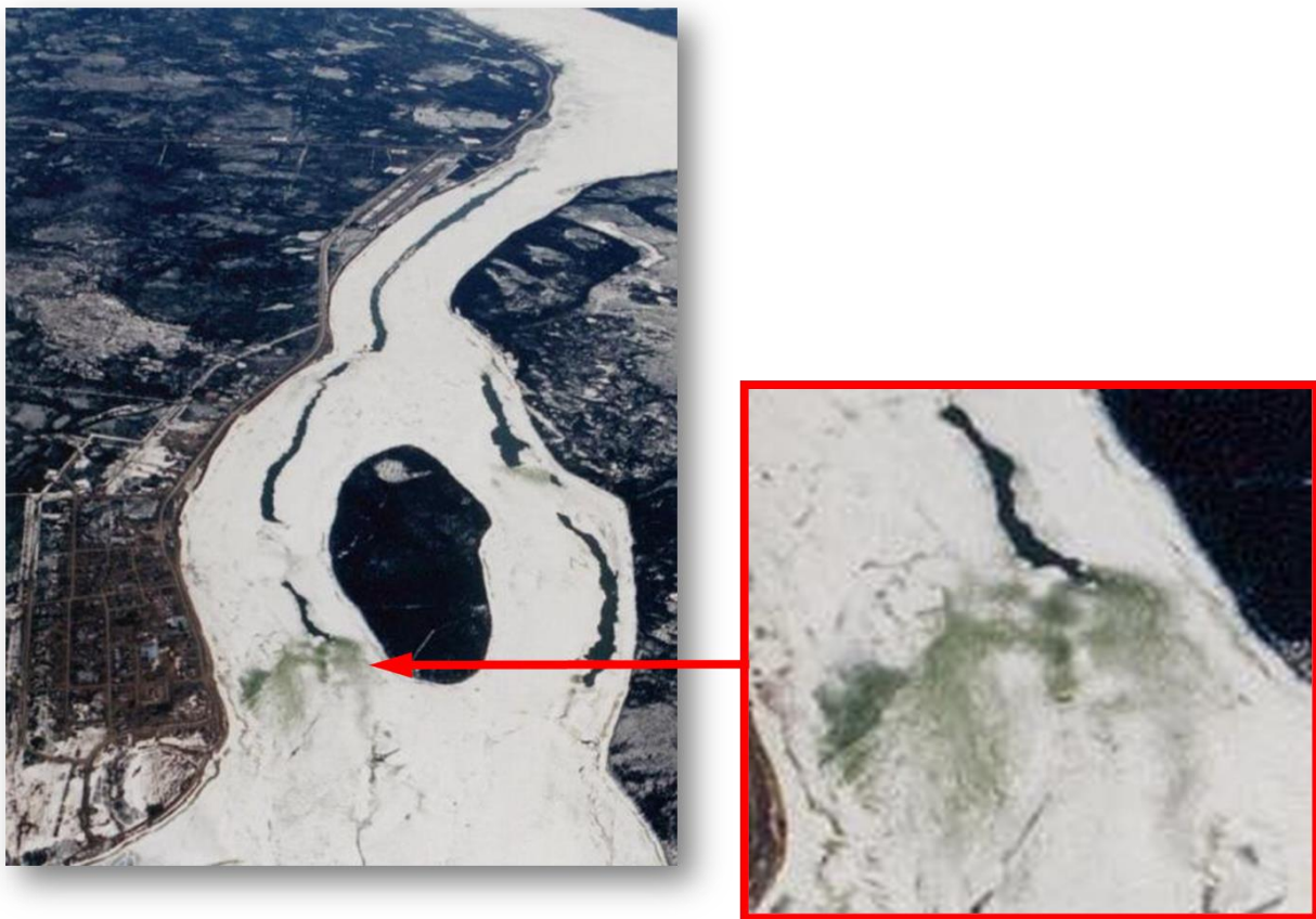
Figure 2.13 Dynamic breakup of river ice with rising water level along thalweg (photo by F. Hicks) When there is a sudden increase in air temperature or when there is a rainfall event that causes the snowpack to quickly melt and the hydrograph of a river to increase sharply, the dynamic break-up is far more likely to occur. Dynamic break-up may also be influenced or caused by additional variables, such as increasing releases from hydropower plants, dams, or reservoirs.
