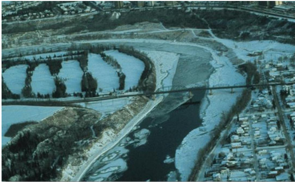
Figure 2.5 Bridging process starting at river bends and constricted areas (photo by R. Gerard, University of Alberta)
