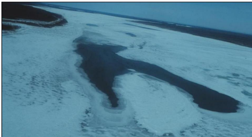
Figure 2.11 Thermal break-up of ice cover because of development of open water leads (photo by F. Hicks)
