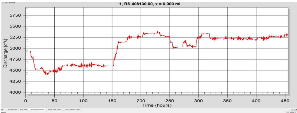
Figure 8.6 Hydrograph view for transient (unsteady) solution for open water case of Missouri River on River1D.
