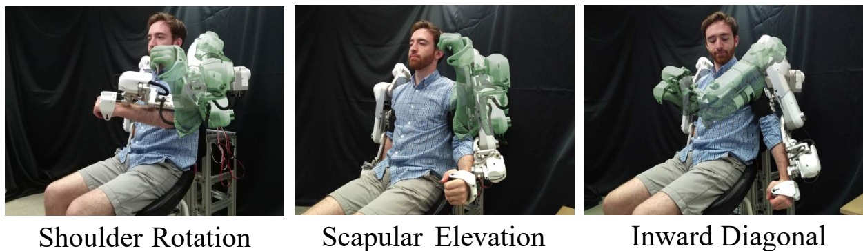
Figure 2.7: Participants performed a set of six coordinated motions during training, and in this thesis we analyze the impact of gravity compensation on a subset of three movements, which involve different levels of effort and shoulder coordination. Specifically, shoulder rotation, scapular elevation, and across-the-body inward diagonal motion.
