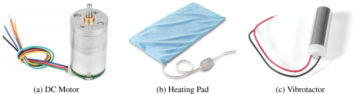
Figure 3.3: Different Commercial off the Shelf Items used for the GAINS-Boot testbed device for DPN.
