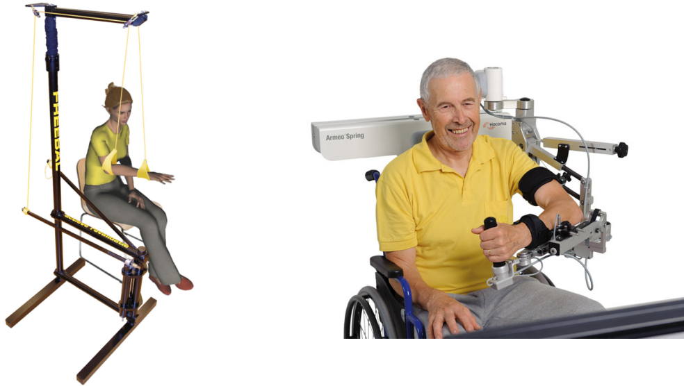
Figure 1.2: The Freebal gravity compensation system (left) generates an upward force via inertia-free ideal-spring mechanism [2]. The Armeo Spring (Right) uses varied spring mechanism to help counteract the effect of gravity via gravity compensation [3,4].
