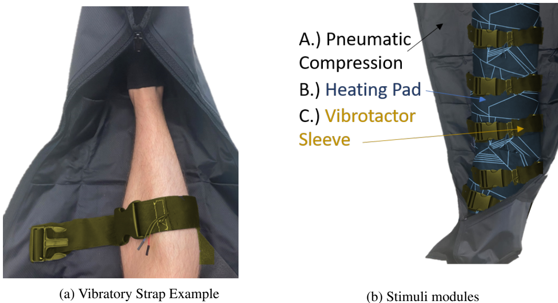
Figure 3.6: On the left is an example of the strap attached around the leg inside of the pneumatic compression boot. GAINS-Boot example stimuli testbed device. This image shows a concept of all three stimuli, labeled above, across the entirety of the shank and foot(right).
