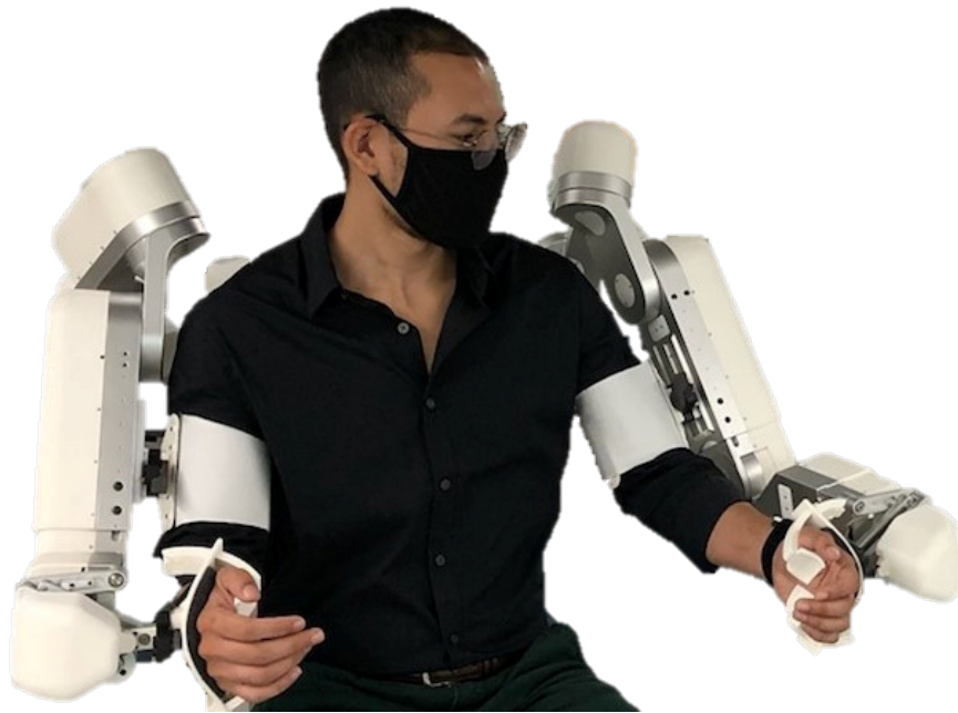
Figure 1.1: Harmony exoskeleton, a bimanual, 14-DOF upper body exoskeleton provides gravity compensation of arm and exo weight during varied arm movements for participants with chronic stroke [1].
