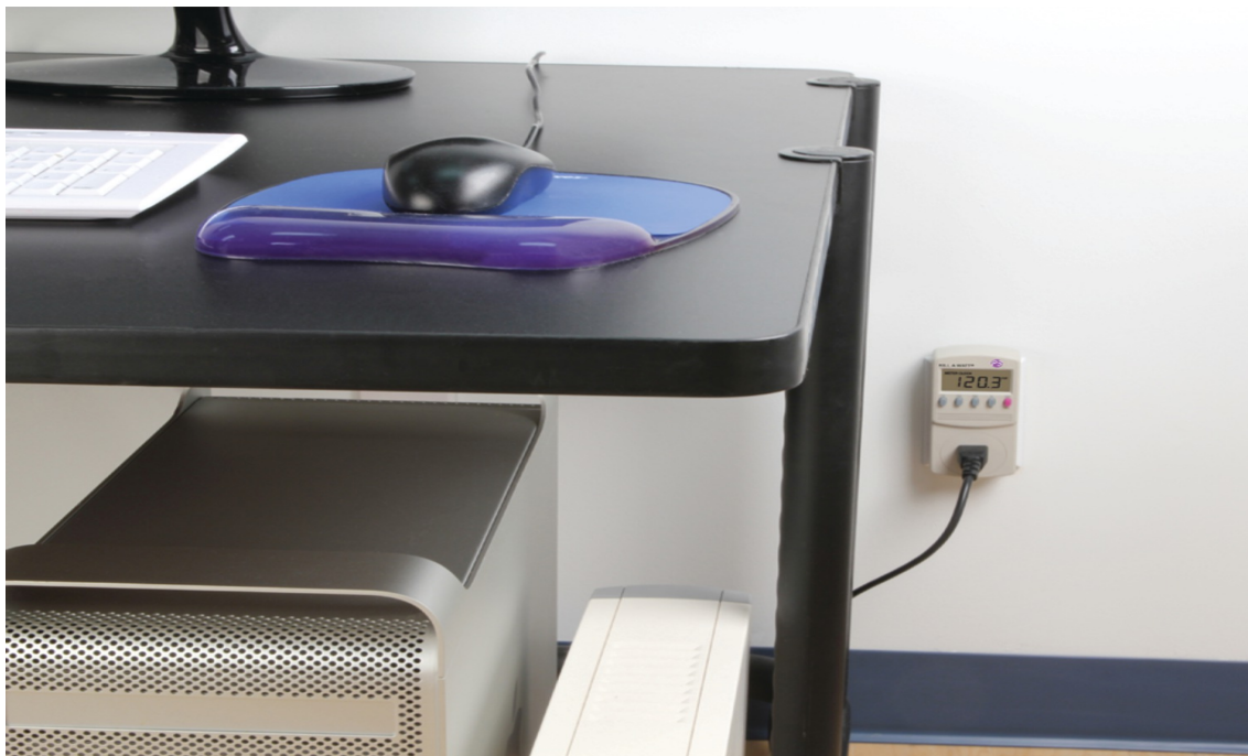
Figure 6.3: A Kill A Watt, P4400 installed as a smart meter captures the power consumption of the monolithic system.
