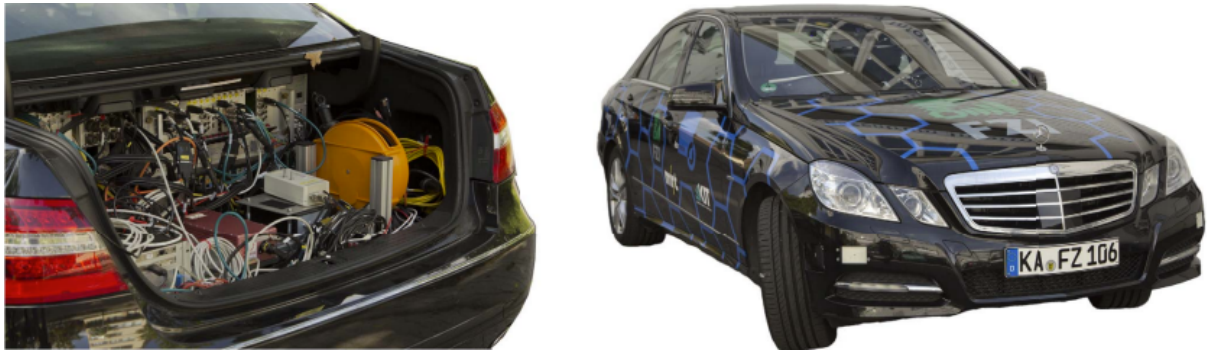
Figure 5.1: BerthaOne robotic vehicle depicting computing hardware configuration [1].
