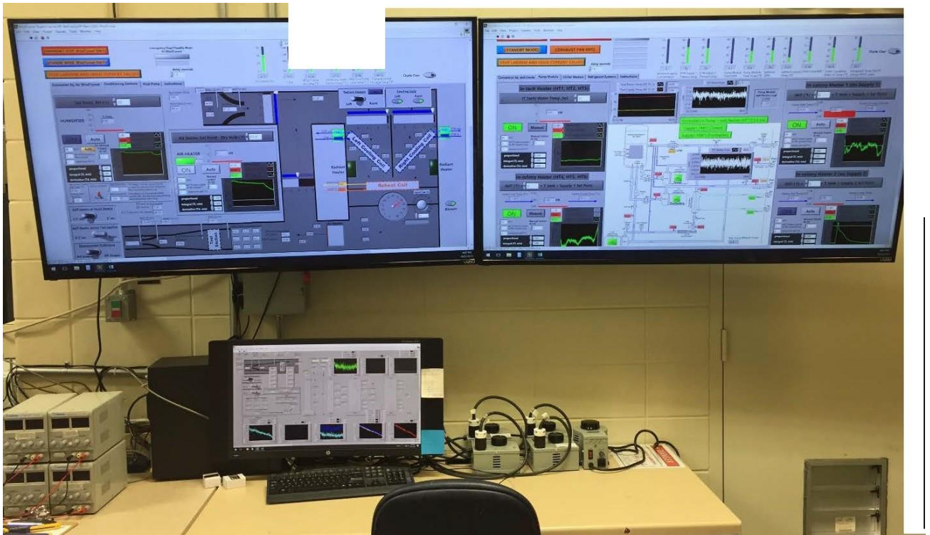
Figure 4.8: LabVIEW data acquisition and computer control system
