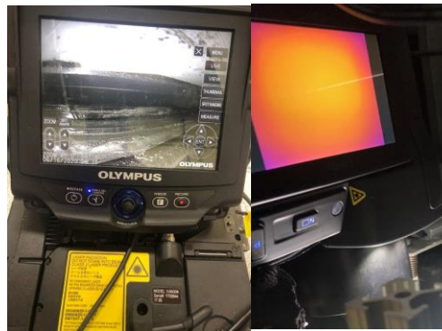
Figure 4.7: Photographic image of the visualization sensors used in the current study. (a) High Resolution Charged Couple Device (HR CCD) camera and (b) Infrared (IR) camera.
