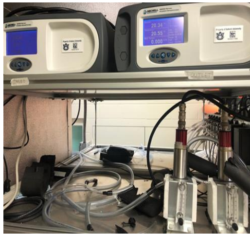
Figure 4.3: image of a dew point pump and sensor device.
