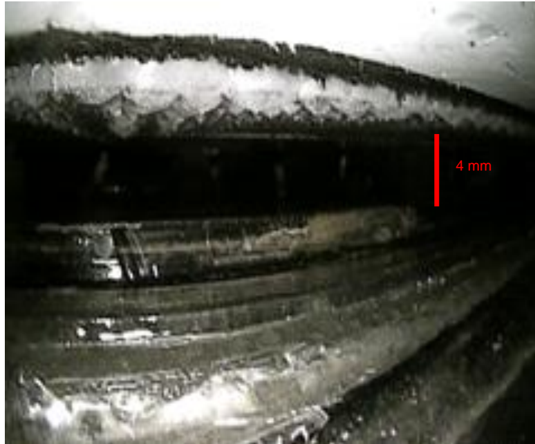
Figure 4.15: Frost thickness measurement
