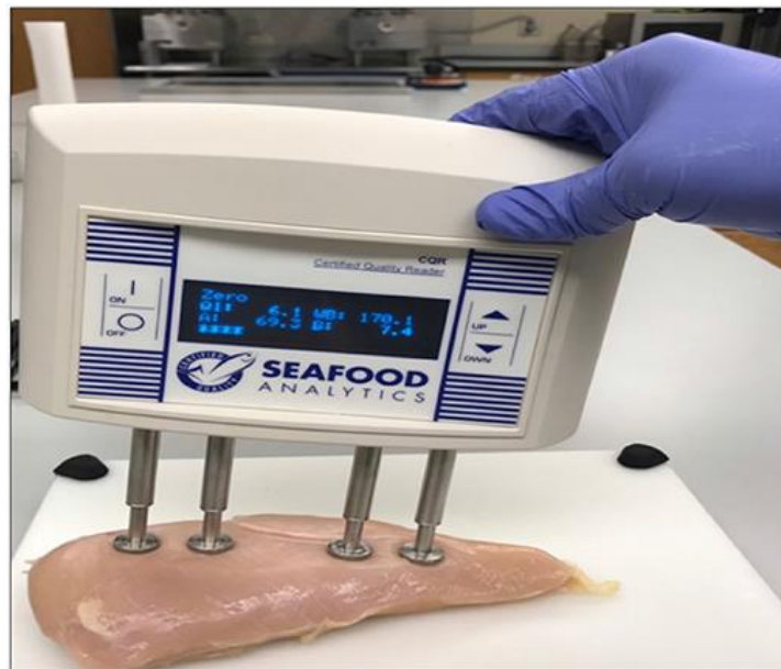
Figure 3-2: Hand-held BIA setup for the classification of fillets based on different myopathic conditions
