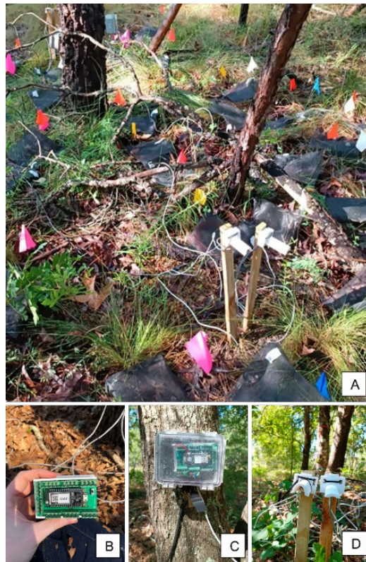
Figure 11. Microclimate sensors. A) Microclimate sensors positioned under the tree canopy. B) Microcontroller (Particle Boron, Particle Industries, Inc., San Francisco CA). C) Microcontroller in rain shield settled on the tree bark. D) Air temperature (VEML 7770) and relative humidity (SHT31) sensors radiation shield. Sensors were placed in duplicate for measurement redundancy.
