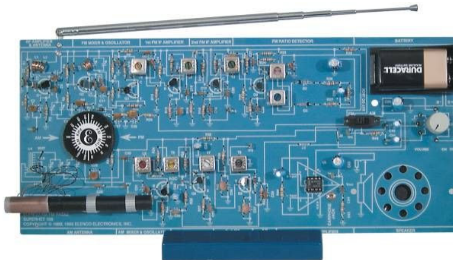
Figure 3.1.1 (a): Assembled AM/FM Trainer kit
