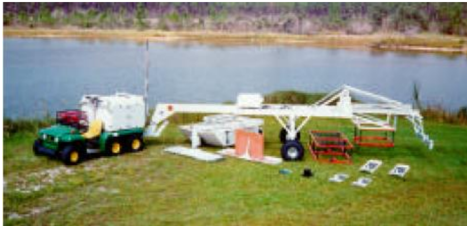
Figure 2.9: AFRL UXO Mapping System [1]
