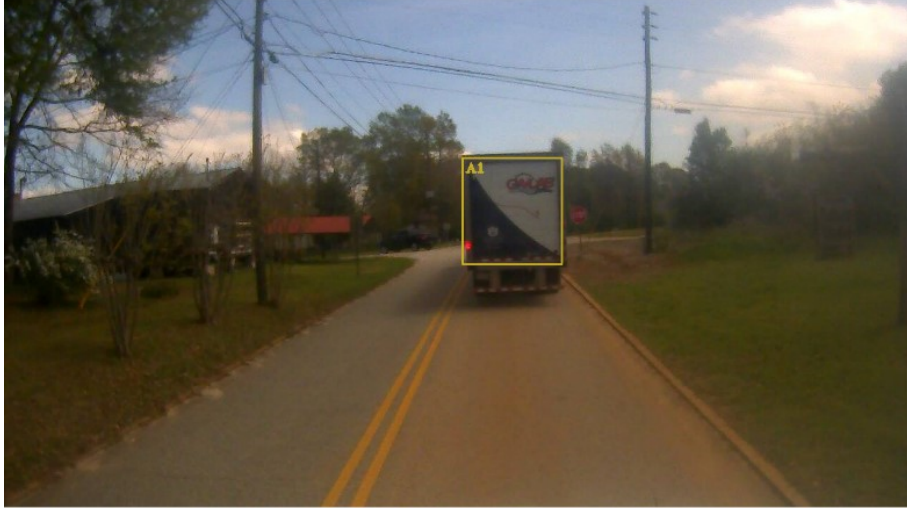
Figure 3.1: Example of Bounding Box Provided by YOLO
