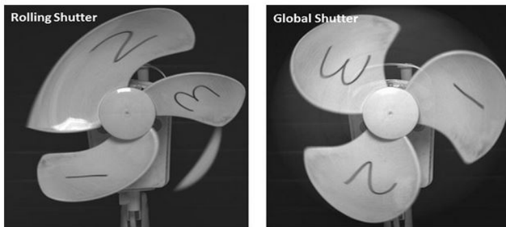
Figure 2.20: Global Shutter and Rolling Shutter [70].
