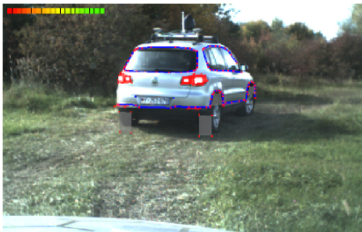
Figure 1.4: Relative Pose Determined using a Camera and Predefined Model [19].
