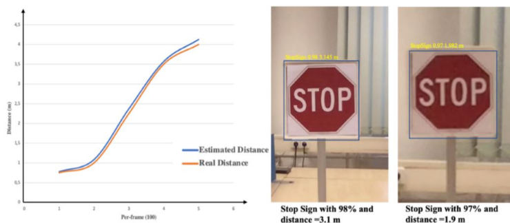
Figure 1.5: YOLO implementation trained to detect and determine range to common street signs [24].
