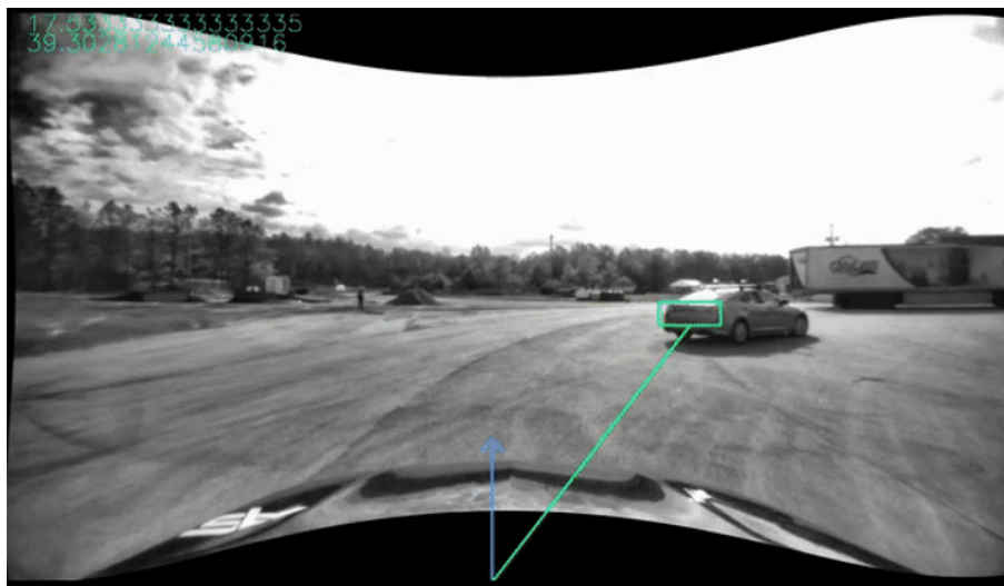
Figure 4.11: Example Output from Monocular RPV Generation Algorithm as Shown by the Visualization Tool.
