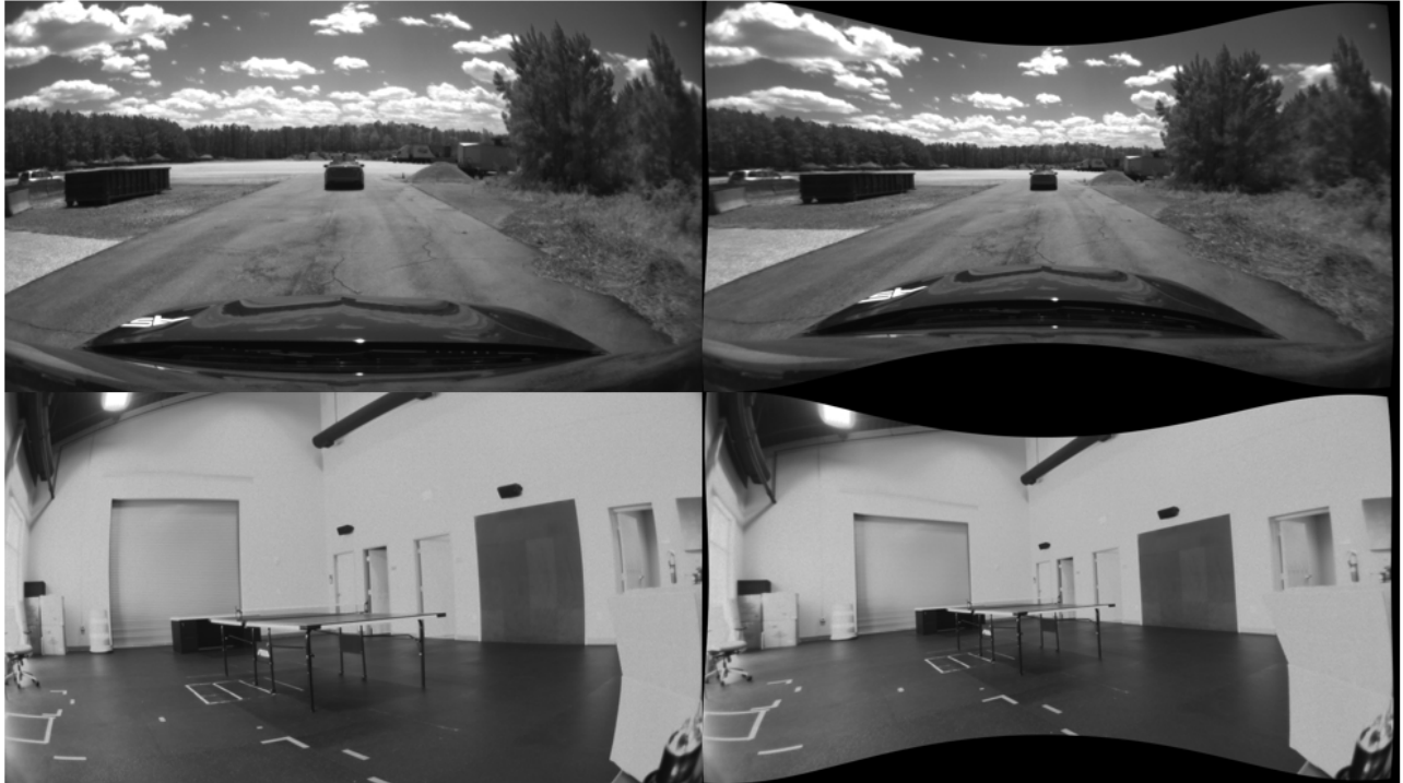
Figure 2.29: Difference between Calibrated and Uncalibrated Images.
