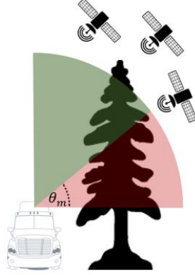
Figure 1.1: Depiction of blocked satellites which would otherwise be viable for a GPS solution.
