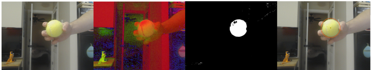
Figure 2.49: Simple HSV based object detector. From left to right: Original Image, HSV Image, Filtered Image (Binary Threshold), Largest Contour (with bounds and centroid annotated).
