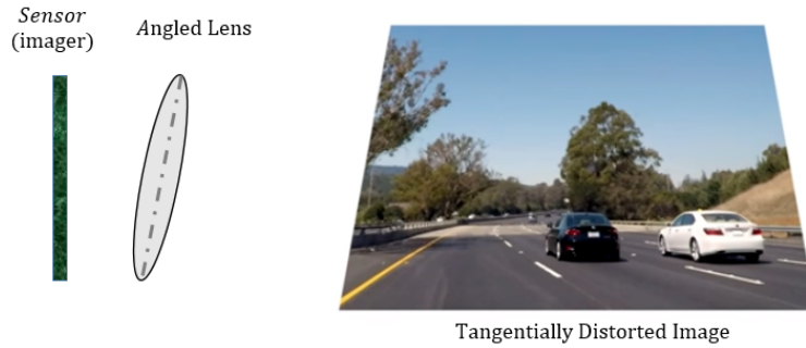
Figure 2.28: The Cause and Effect of Tangential Distortion
