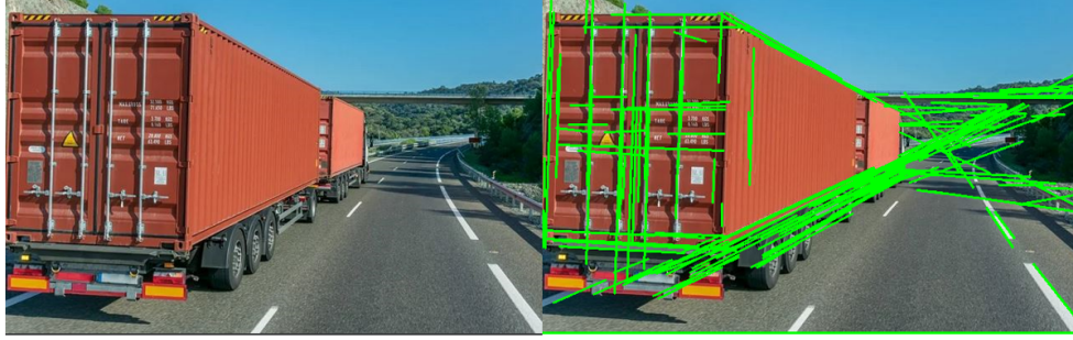
Figure 2.39: Probabilistic Hough Transform Function (OpenCV) applied to the canny edge detection algorithm from Figure 2.37.
