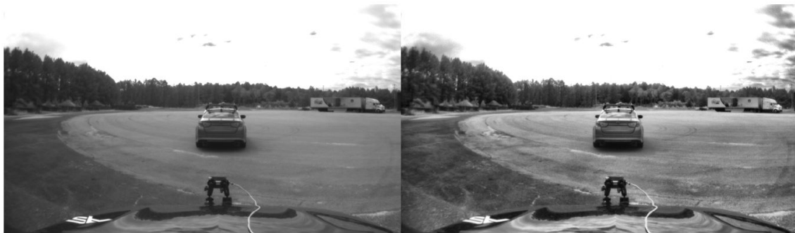
Figure 4.4: Original Image (left), CLAHE Algorithm Applied (right).
