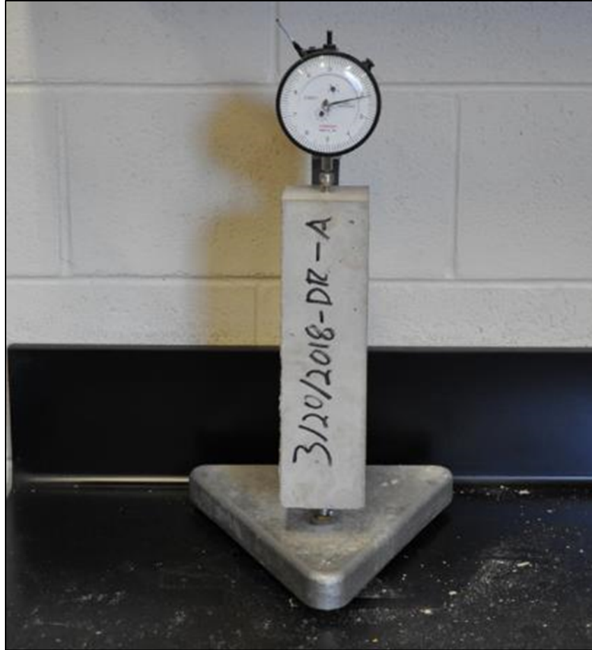
Figure 4-7: Standard length comparator used to measure drying shrinkage
