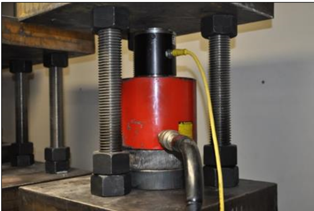
Figure 4-11: Setup of hydraulic ram and load cell on creep testing frame
