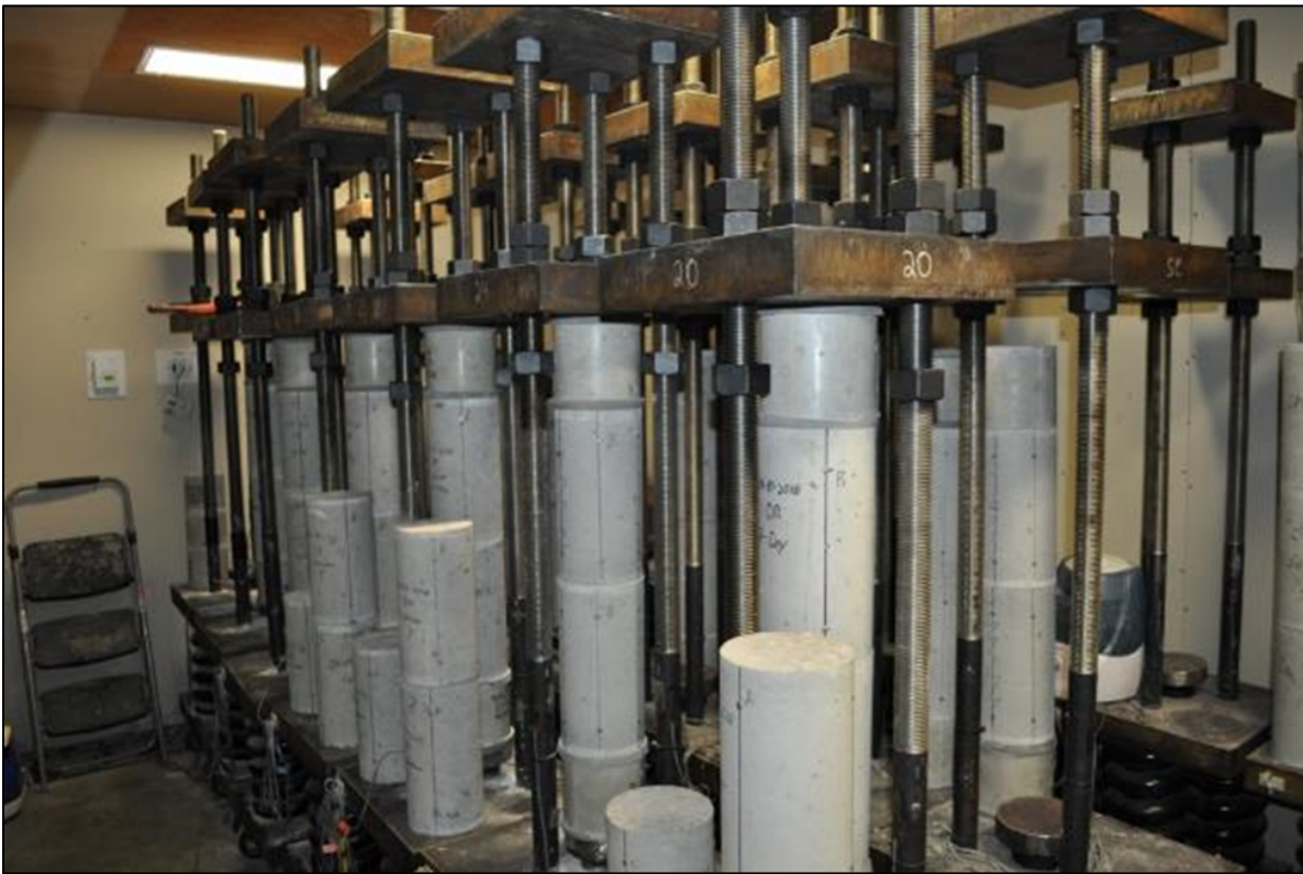
Figure 4-10: Creep testing room
