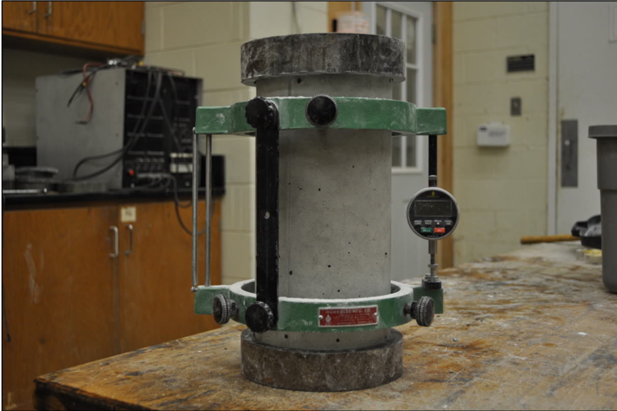
Figure 4-6: Compressometer used to test modulus of elasticity
