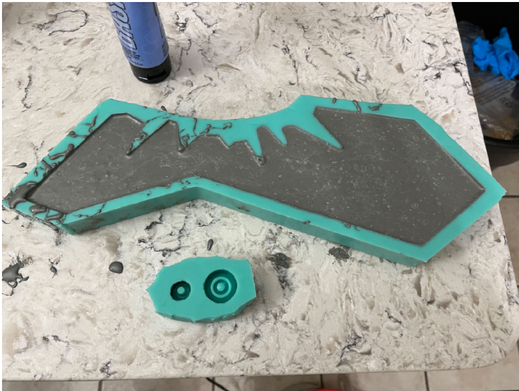
Figure 70: Pouring Resin-cement Mixture.
