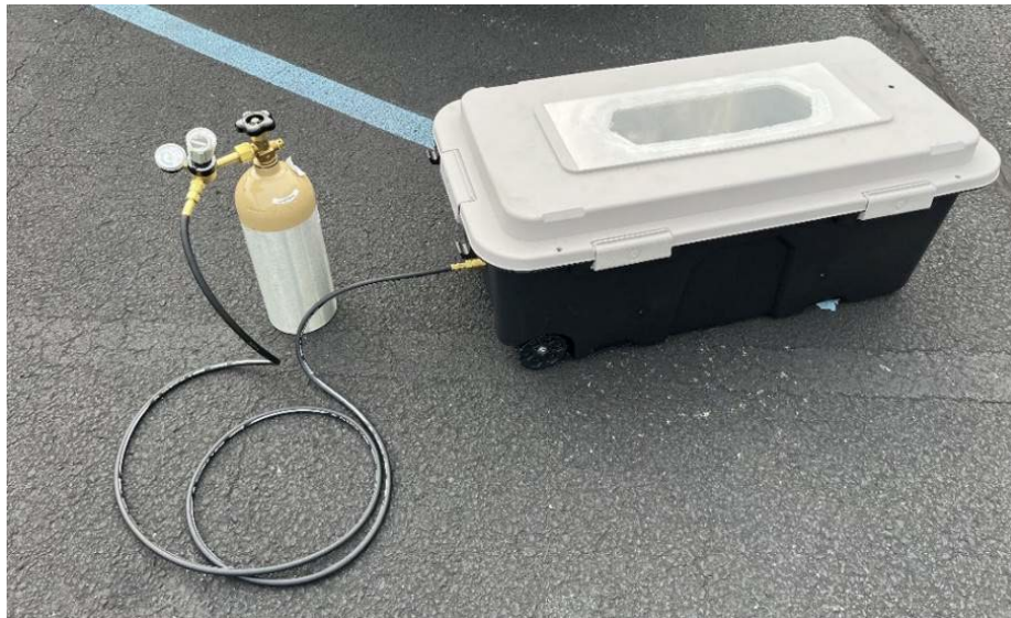
Figure 3.6. A constructed euthanasia chamber with an attached five-gallon carbon dioxide tank and regulator. Not pictured is the box trap inside of the chamber that can be placed without physically translocating the animal.
