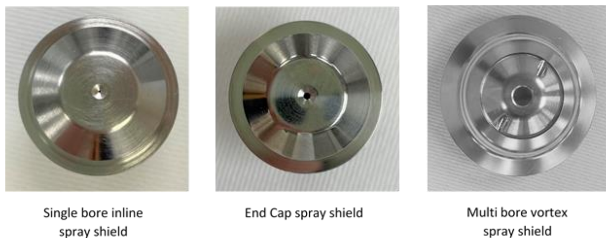
Figure 3.2. Pictures of various nanospray shields used in this work.
