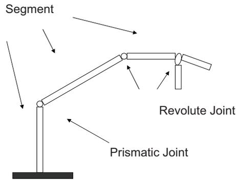
Figure 2.1: Robot Manipulator identifying segments and joints.
