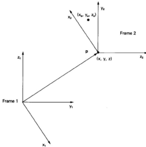
Figure 4.3: Displaced Reference Frames in the Same Space, ref. Klafter [10].
