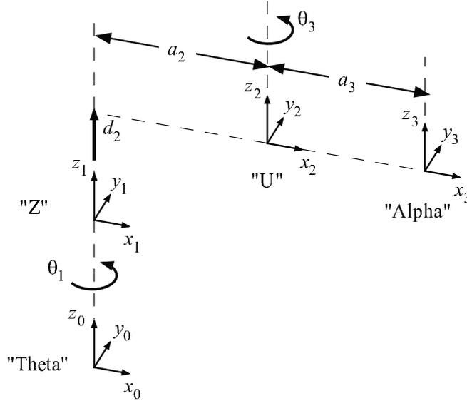
Figure 4.6: Establishing Link Coordinate Frames for the GMF A-510 Robot, ref. Hung [8].
