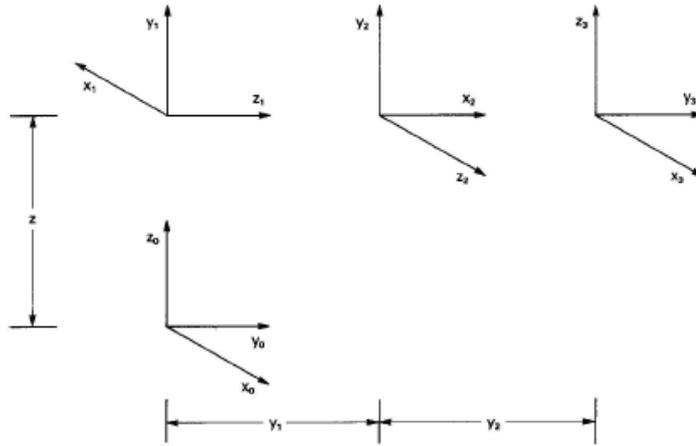
Figure 4.4: Alignment of Reference Frames Example, ref. Klafter [10].
