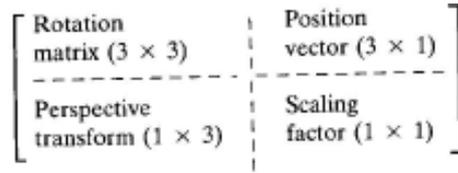
Figure 4.2: Homogeneous Transformation Matrix I, ref. Klafter [10].
