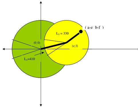
Figure 5.1: Algebraic Model: Top View of GMF A-510 Robot
