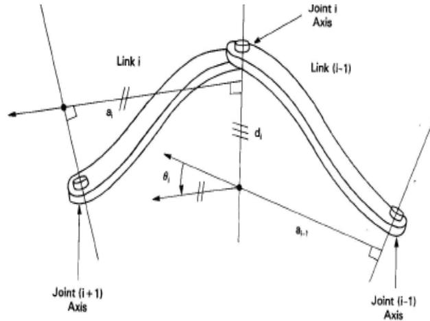
Figure 4.5: Establishing Link Coordinate Reference Frames, ref. Lee [14].
