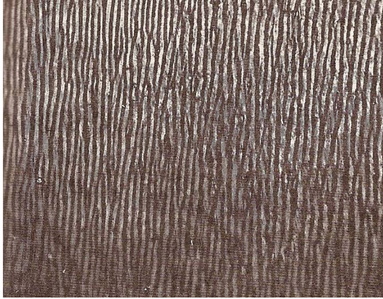
Figure 2.7 Shear bands in dried films of 15% PBLG + dioxane at high shear rate (Kiss and S.Porter 1998).
