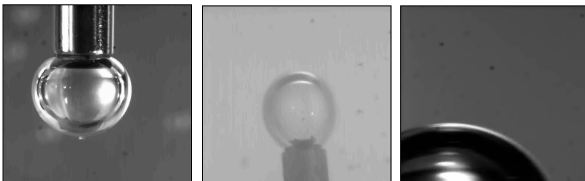
Figure 3.2: Examples of stationary bubbles. a.) Stationary bubble on the tip of an inverted needle. b.) Stationary bubble on the tip of an upwardly oriented needle. c.) Higher magnification image of the surface of a stationary bubble.
