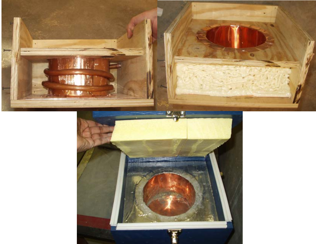
Figure 3-10: Setting test box construction
