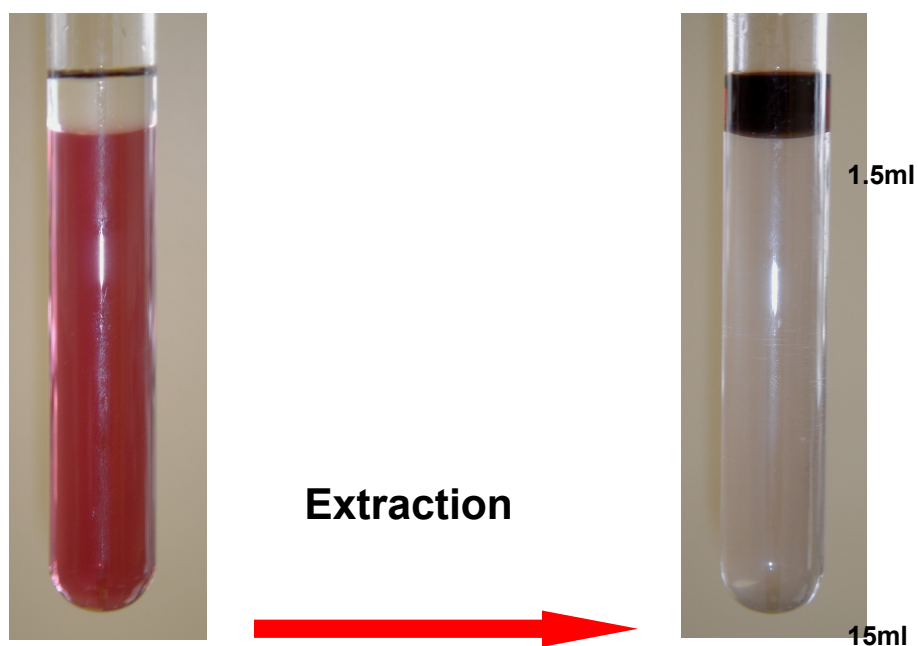
Figure 5-S3: Digital images illustrating the effective extraction of Au nanoparticles from an aqueous \beta -D glucose solution into a hexane phase via ligand exchange from \beta -D glucose to dodecanethiol. These images display the generation of highly concentrated dodecanethiol capped Au nanoparticle dispersions in hexane.
